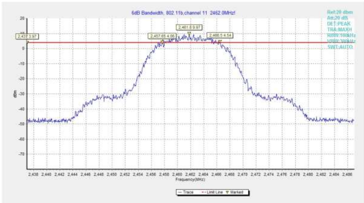
Fig.A.4.3 Occupied 6dB Bandwidth (802.11b, Ch 11)
