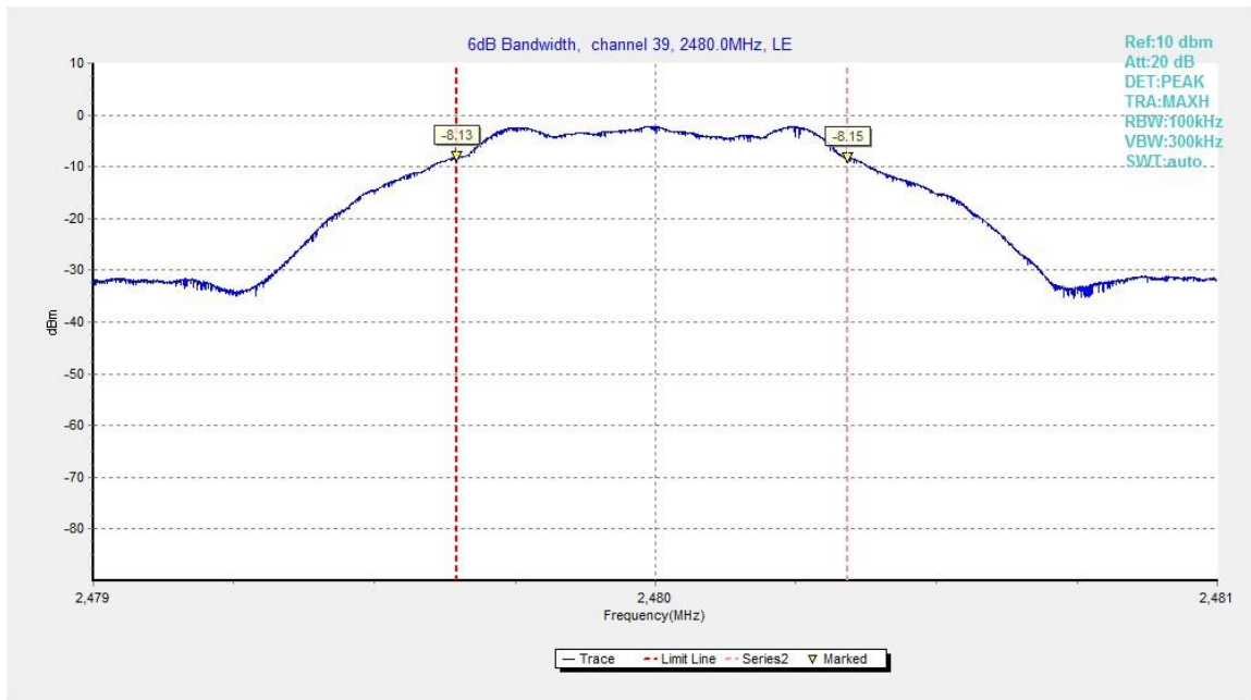
Fig.22. 6dB Bandwidth: GFSK, 2480 MHz
