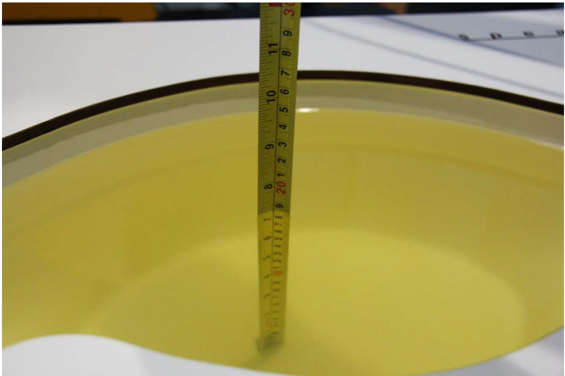
Picture 7-5: Liquid depth in the Flat Phantom(2450MHz)
