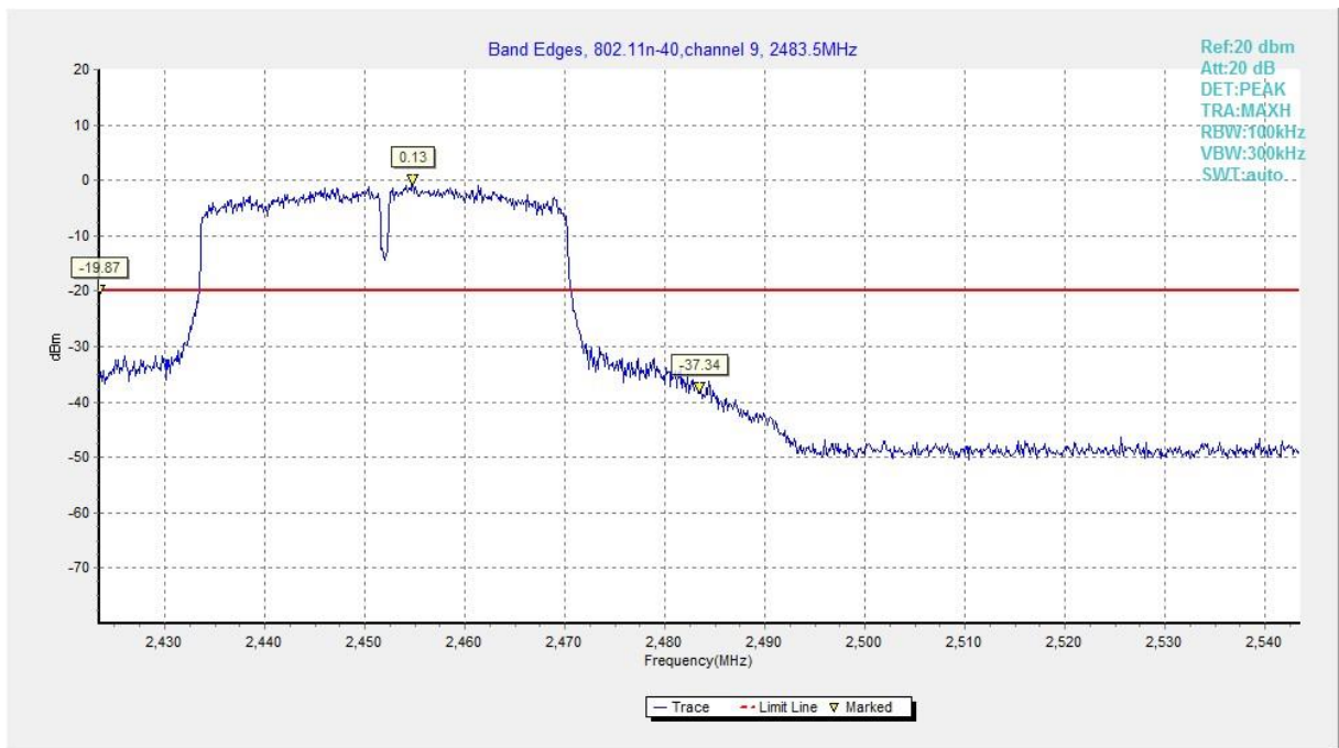
Fig.A.5.8 Band Edges (802.11n-HT40, Ch 9)
