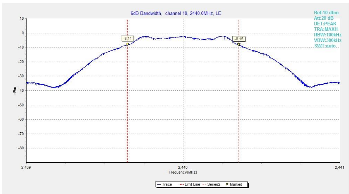
Fig.21. 6dB Bandwidth: GFSK, 2440 MHz
