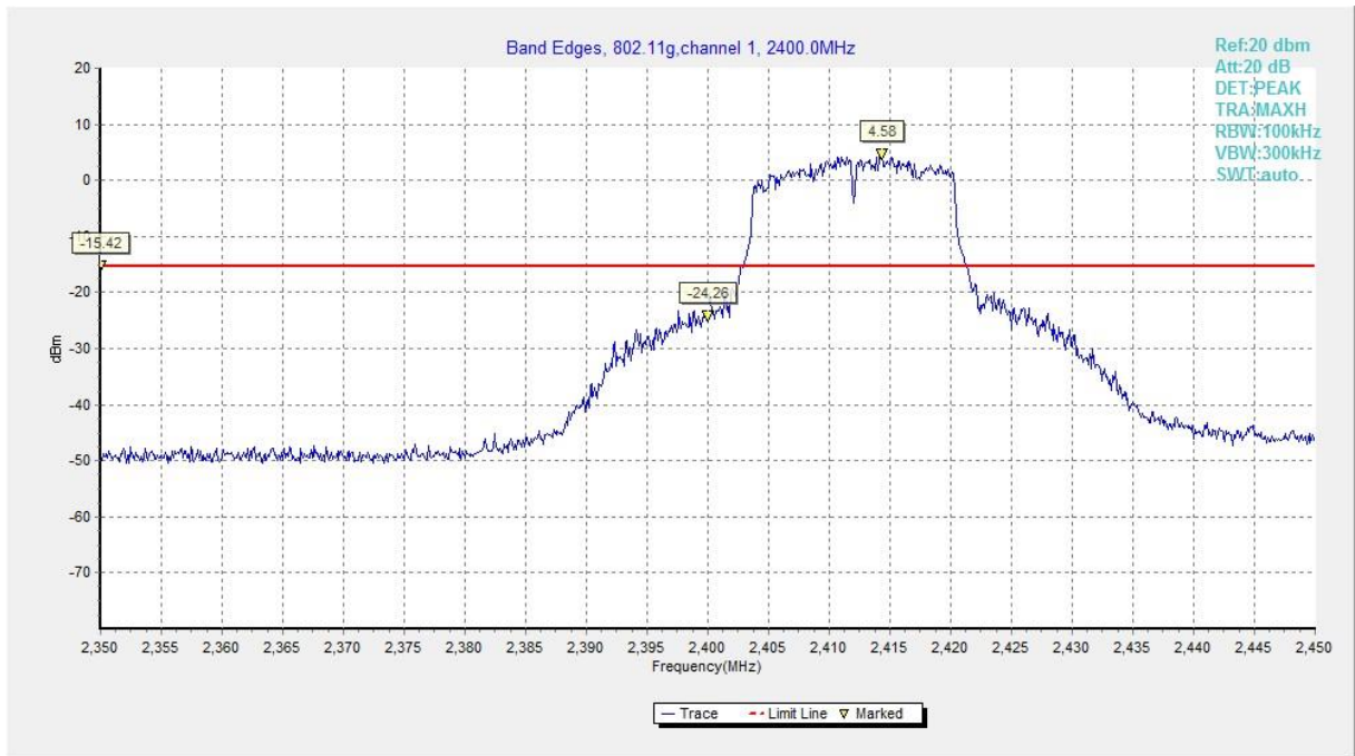
Fig.A.5.3 Band Edges (802.11g, Ch 1)
