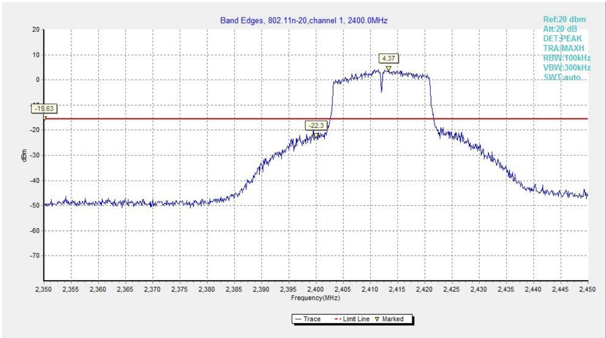
Fig.A.5.5 Band Edges (802.11n-HT20, Ch 1)
