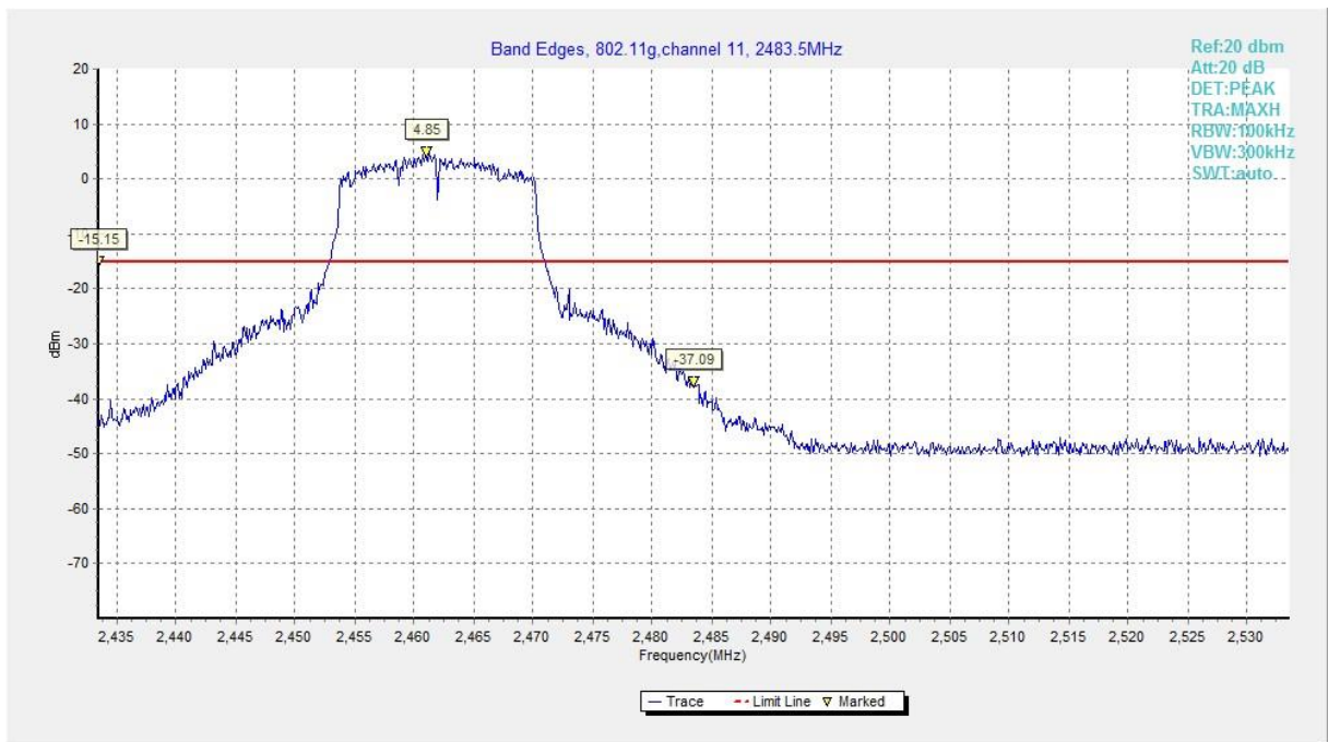
Fig.A.5.4 Band Edges (802.11g, Ch 11)
