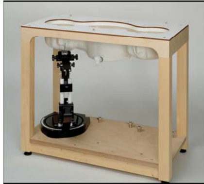
Picture C.10: SAM Twin Phantom
