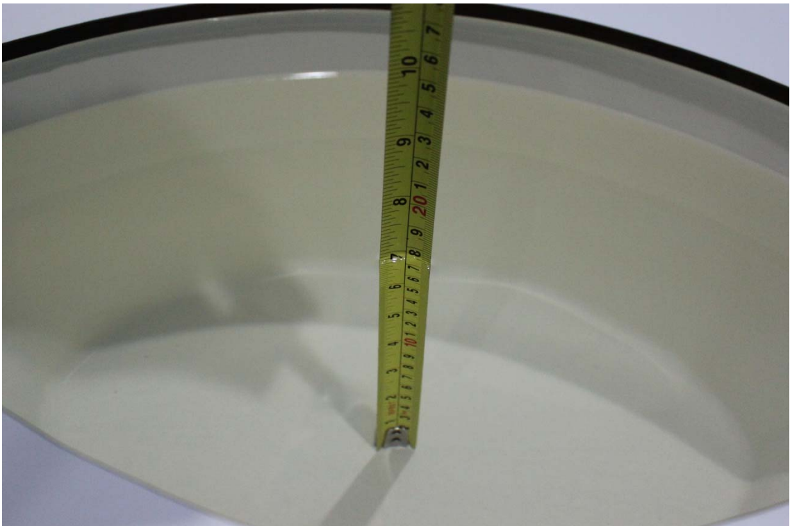
Picture 7-14 Liquid depth in the Flat Phantom (5GHz)
