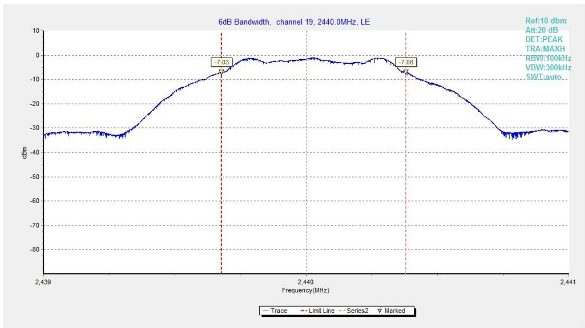
Fig.21. 6dB Bandwidth: GFSK, 2440 MHz
