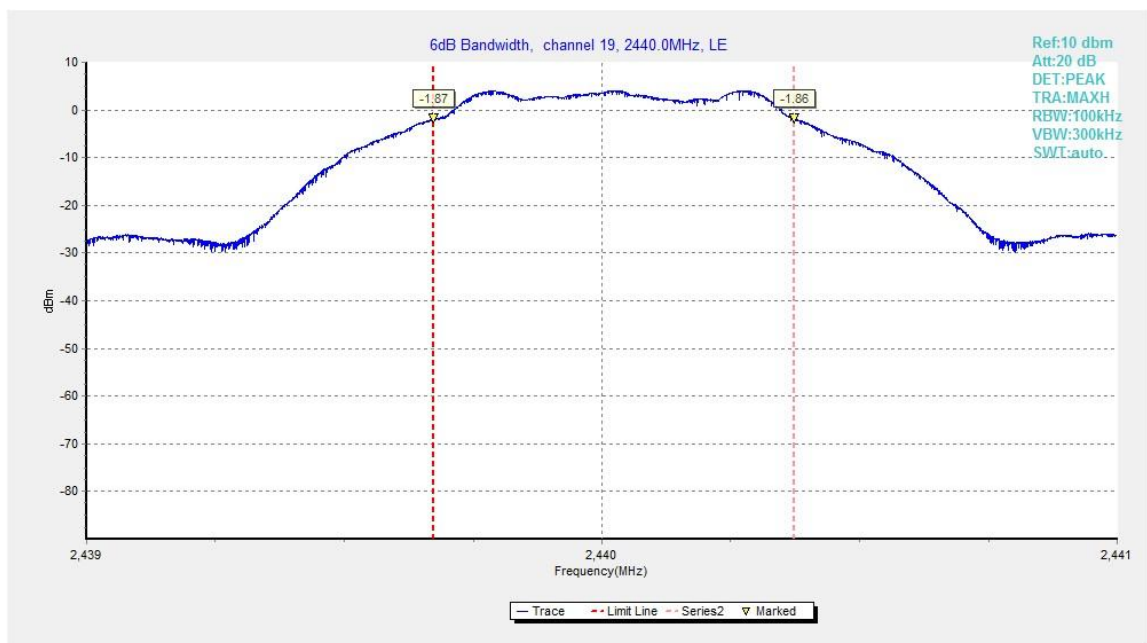
Fig.21. 6dB Bandwidth: GFSK, 2440 MHz
