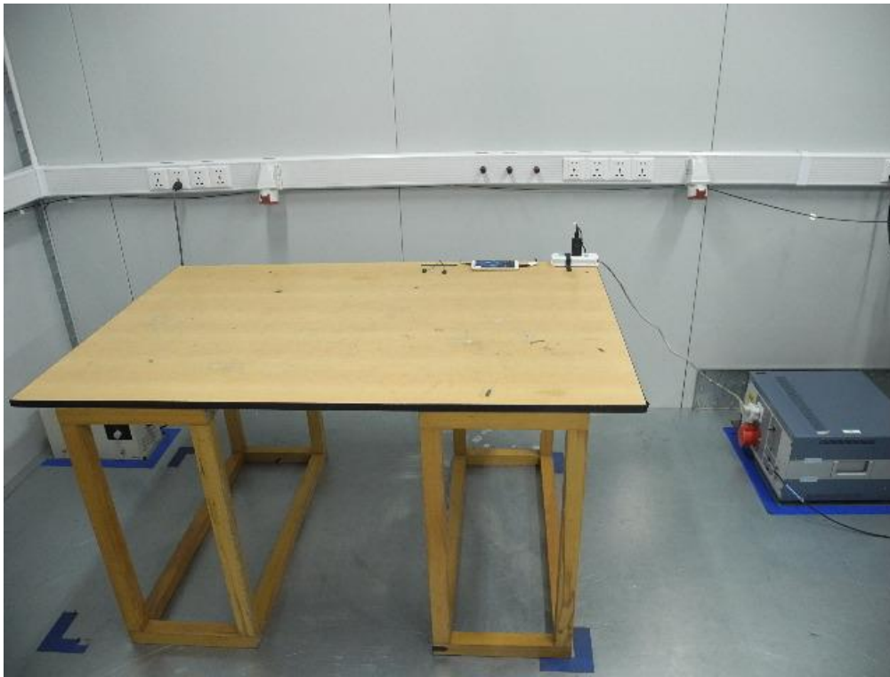
AC Conducted Emission Test Setup -Front
