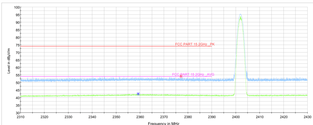
Fig.62. Frequency Band Edges: 8DPSK, Channel 0, 2.31 GHz - 2.45GHz
