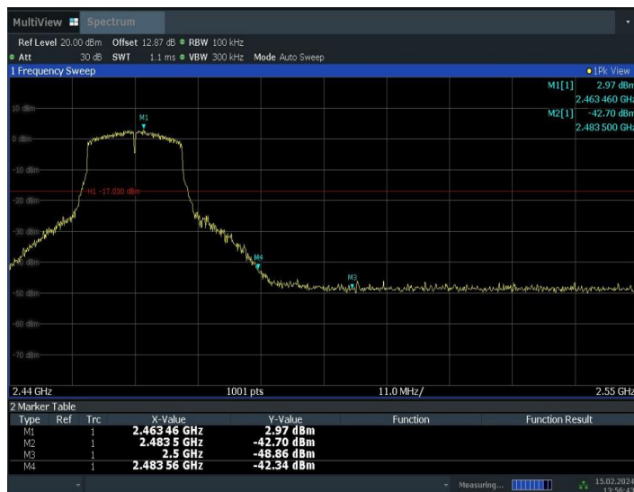
Fig.A.5.4 Band Edges (802.11g, Ch 11)
