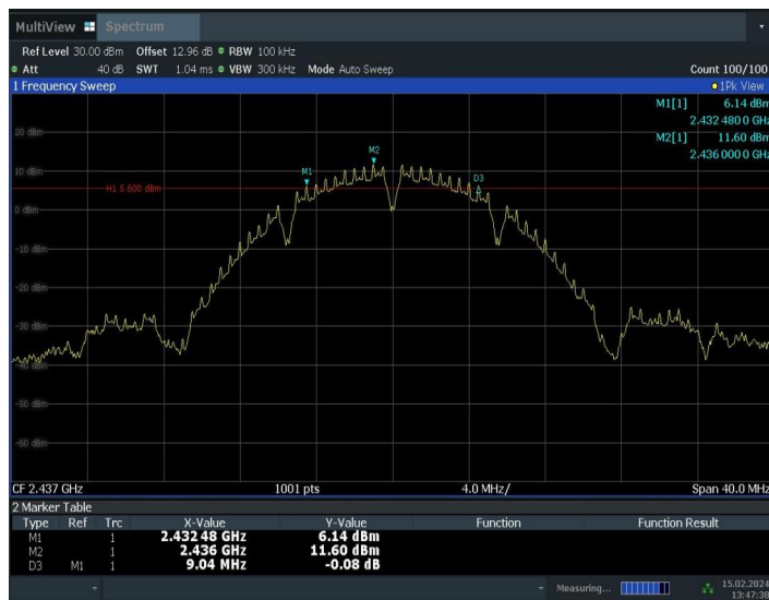
Fig.A.4.2 DTS Bandwidth (802.11b, Ch 6)
