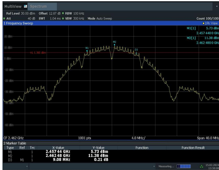
Fig.A.4.3 DTS Bandwidth (802.11b, Ch 11)
