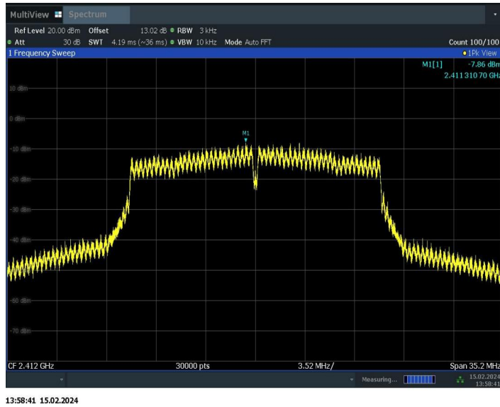
Fig.A.3.7 Power Spectral Density (802.11n-HT20, Ch 1)
