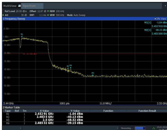
Fig.A.5.8 Band Edges (802.11n-HT40, Ch 9)
