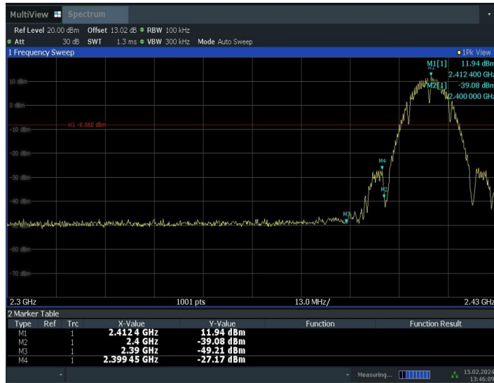
Fig.A.5.1 Band Edges (802.11b, Ch 1)
