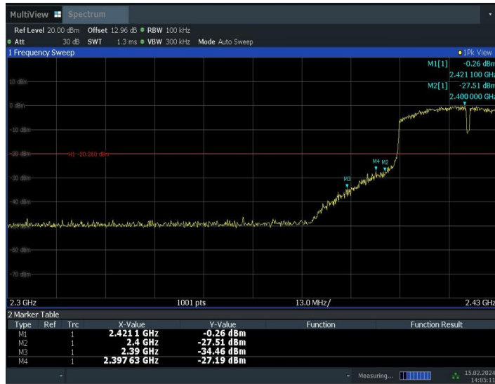
Fig.A.5.7 Band Edges (802.11n-HT40, Ch 3)
