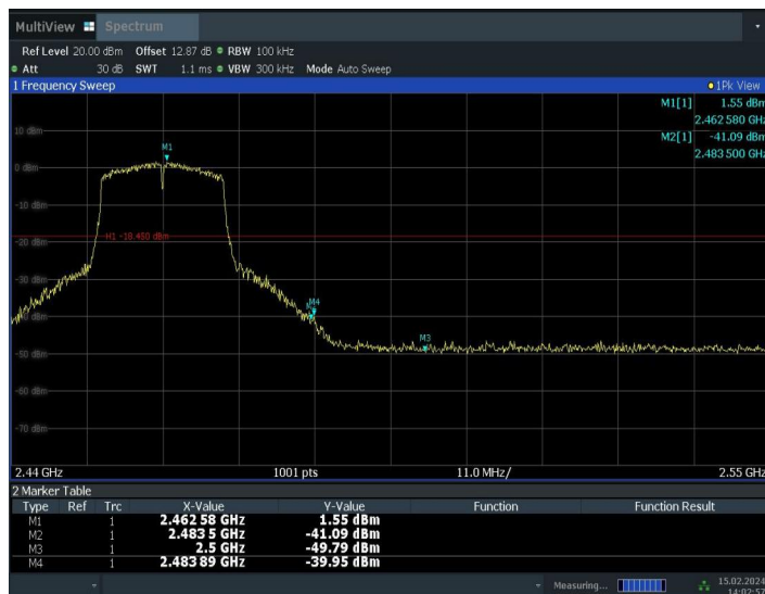
Fig.A.5.6 Band Edges (802.11n-HT20, Ch 11)
