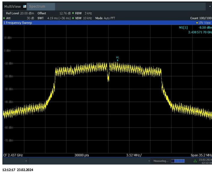
Fig.A.3.8 Power Spectral Density (802.11n-HT20, Ch 6)
