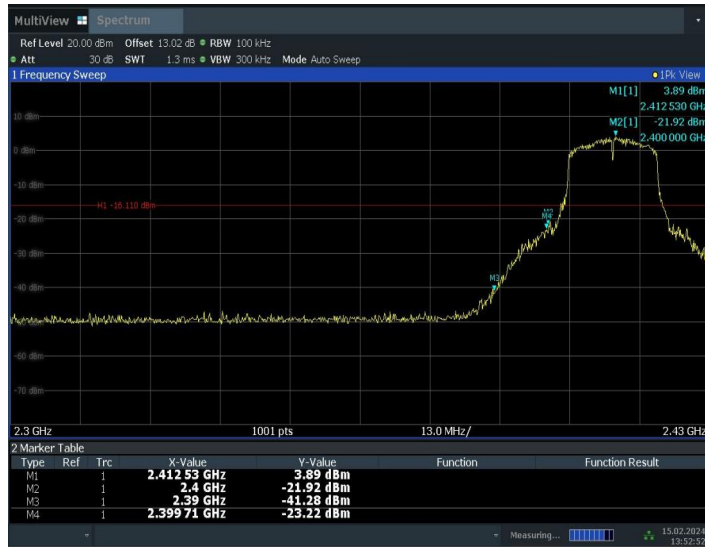
Fig.A.5.3 Band Edges (802.11g, Ch 1)
