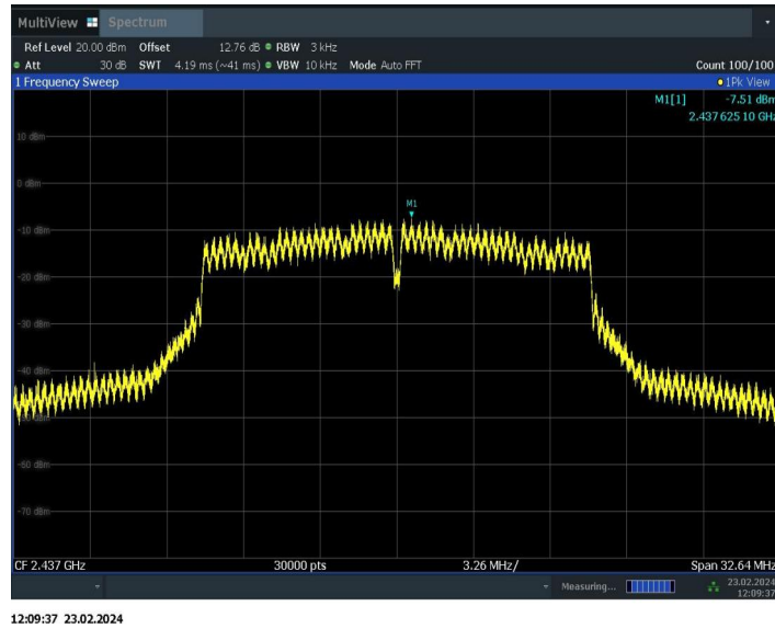
Fig.A.3.5 Power Spectral Density (802.11g, Ch 6)
