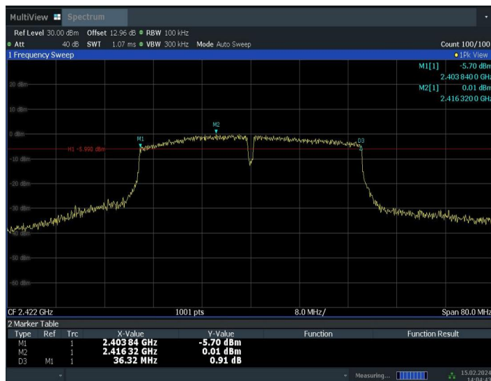
Fig.A.4.10 DTS Bandwidth (802.11n-40MHz, Ch 3)
