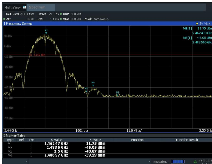
Fig.A.5.2 Band Edges (802.11b, Ch 11)
