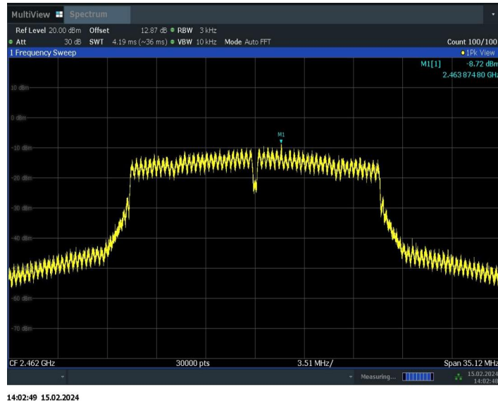
Fig.A.3.9 Power Spectral Density (802.11n-HT20, Ch 11)
