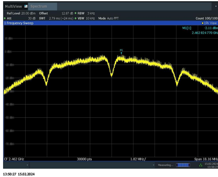
Fig.A.3.3 Power Spectral Density (802.11b, Ch 11)
