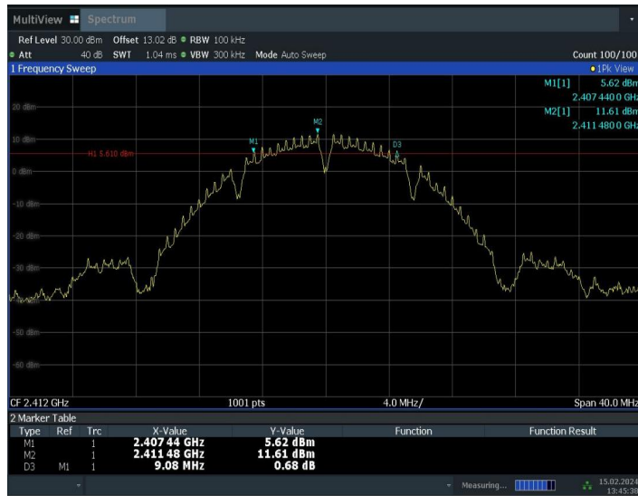
Fig.A.4.1 DTS Bandwidth(802.11b,Ch 1)
