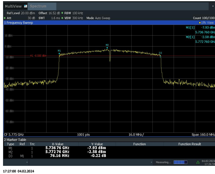
Fig. 9 6dB Emission Bandwidth (802.11ac-VHT80, Ch 155)
