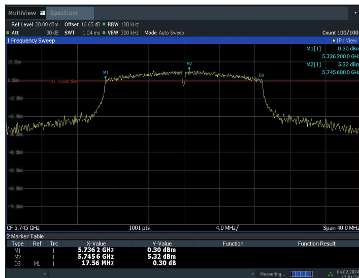
Fig. 4 6dB Emission Bandwidth (802.11ac-VHT20, Ch 149)
