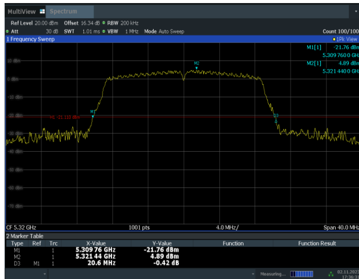
Fig.16 26dB Emission Bandwidth (802.11n-HT20, 5320MHz)
