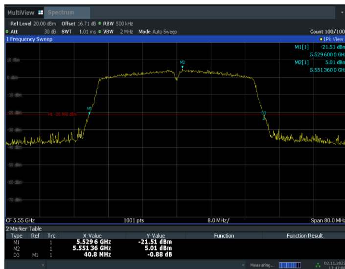
Fig.26 26dB Emission Bandwidth (802. 11ac-VHT40, 5550MHz)
