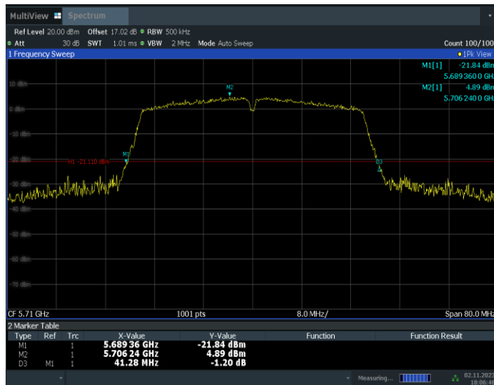
Fig.28 26dB Emission Bandwidth (802. 11ac-VHT40, 5710MHz)
