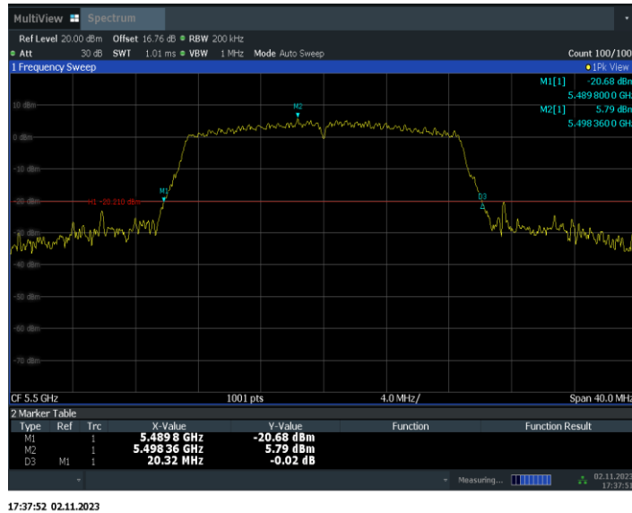
Fig.17 26dB Emission Bandwidth (802. 11n-HT20, 5500MHz)
