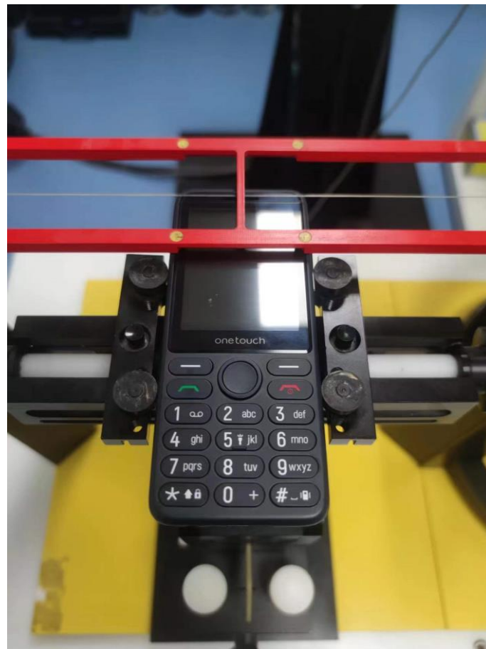
Picture 2: EUT Positioning for RF/T-coil
