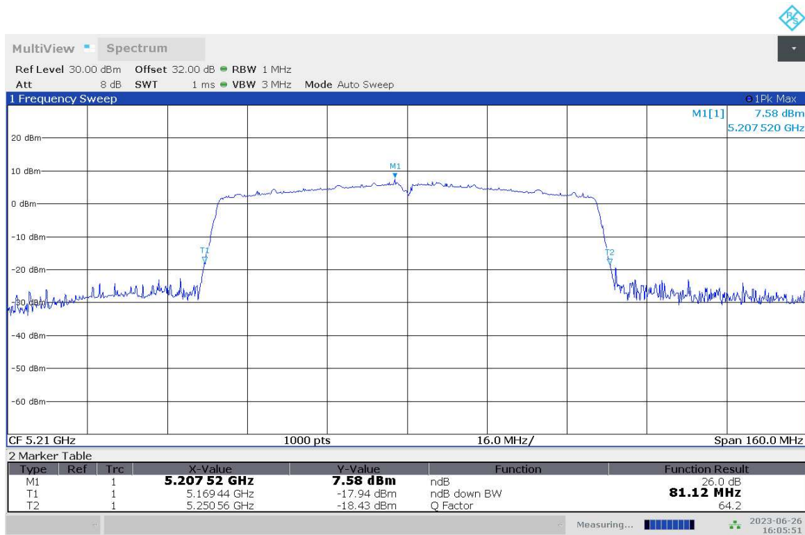
Fig.8 Occupied 26dB Bandwidth (802.11n-HT40, 5230MHz)
