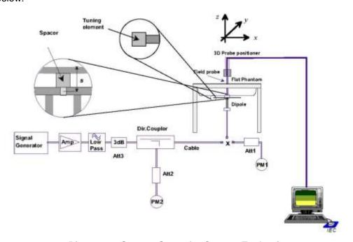
Picture 8.1 System Setup for System Evaluation
