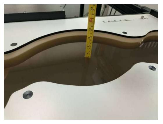
Picture 7-1 Liquid depth in the Flat Phantom
