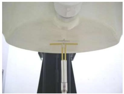
**Picture 8.2 Photo of Dipole Setup**
