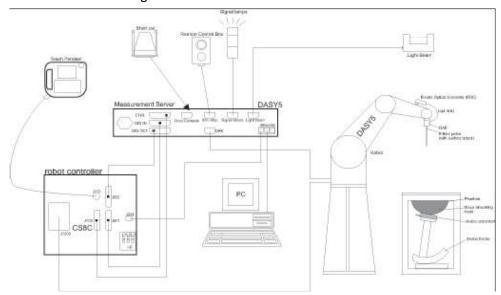
Picture C.1SAR Lab Test Measurement Set-up
