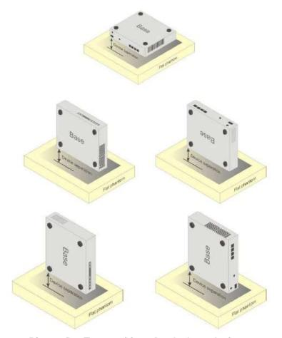
Picture D.2 Test positions for desktop devices
