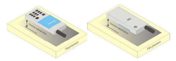
Picture D.1 Test positions for body-worn devices
