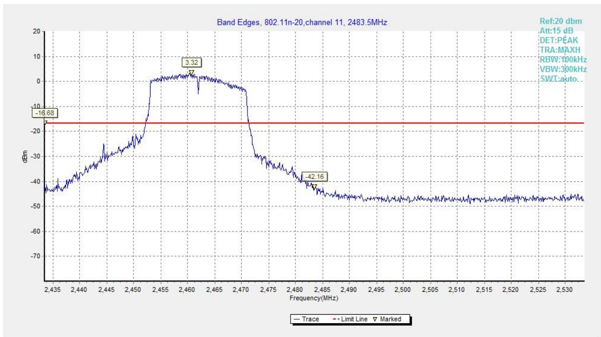
Fig.A.5.6 Band Edges (802.11n-HT20, Ch 11)
