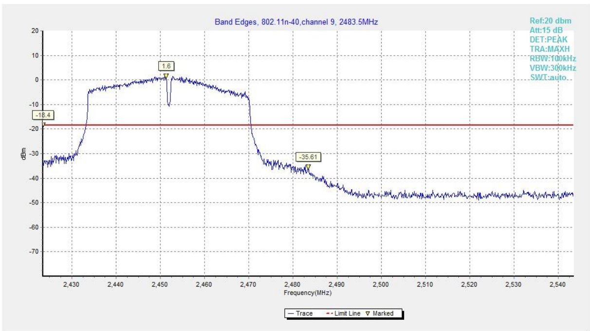
Fig.A.5.8 Band Edges (802.11n-HT40, Ch 9)
