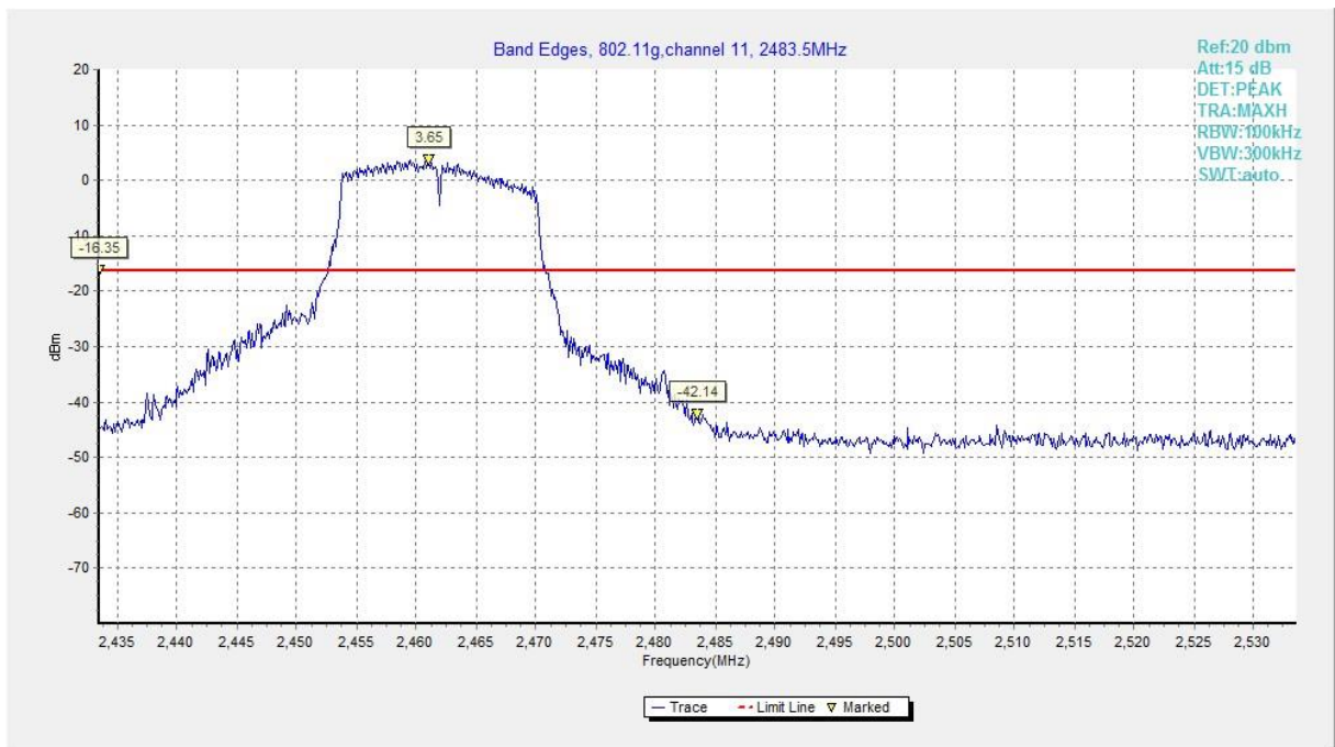
Fig.A.5.4 Band Edges (802.11g, Ch 11)
