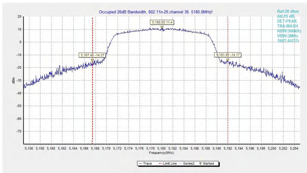
Fig.11 Occupied 26dB Bandwidth (802.11n-HT20, 5180MHz)
