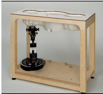
Picture C.10: SAM Twin Phantom
