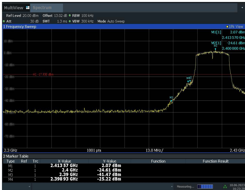
Fig.A.5.5 Band Edges (802.11n-HT20, Ch 1)
