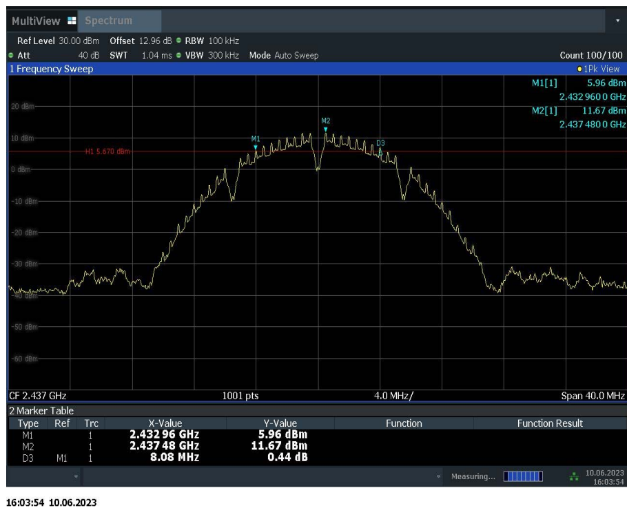
Fig.A.4.2 Occupied 6dB Bandwidth (802.11b, Ch 6)
