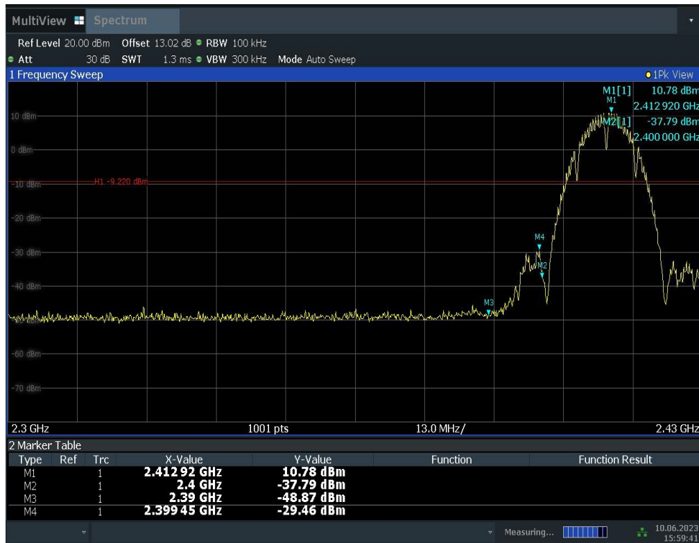
Fig.A.5.1 Band Edges (802.11b, Ch 1)
