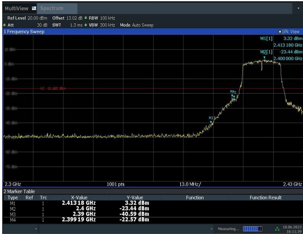
Fig.A.5.3 Band Edges (802.11g, Ch 1)
