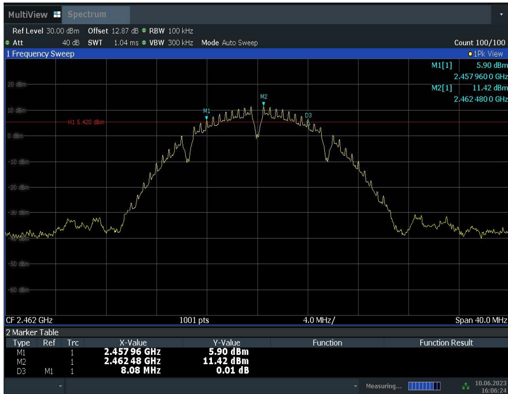
Fig.A.4.3 Occupied 6dB Bandwidth (802.11b, Ch 11)
