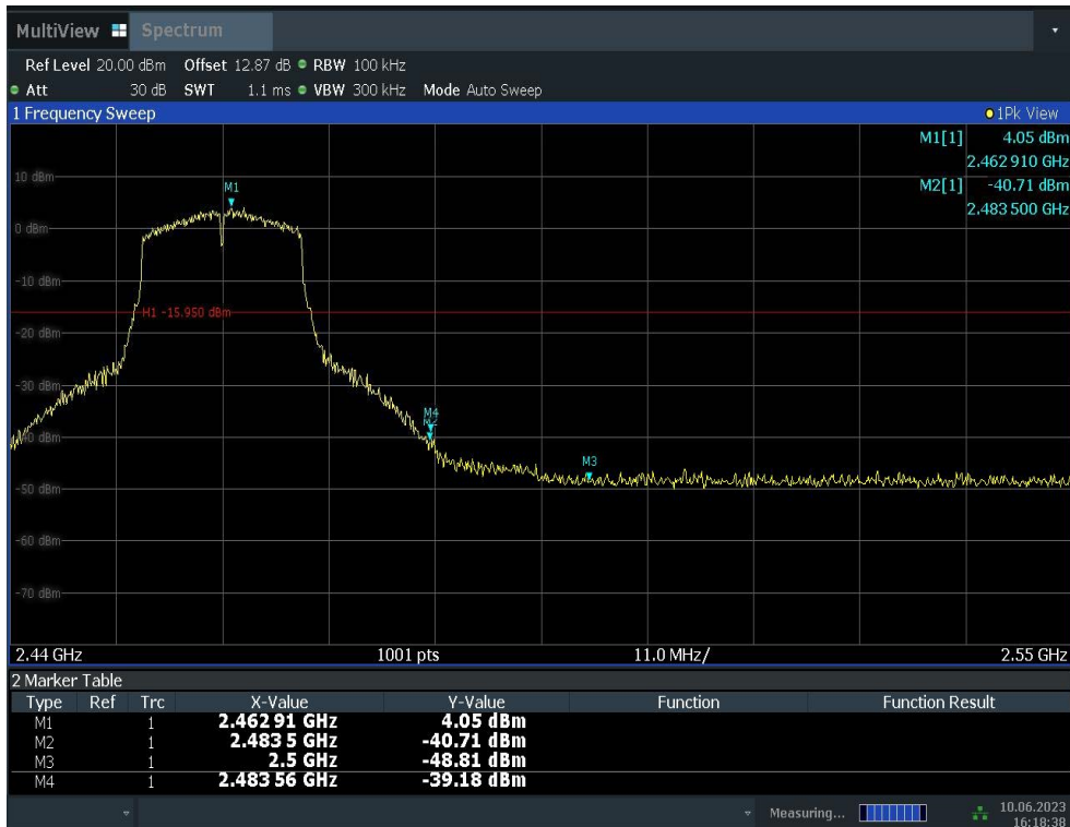
Fig.A.5.4 Band Edges (802.11g, Ch 11)
