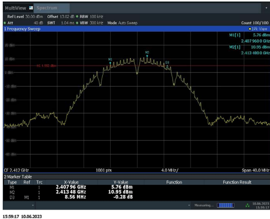
Fig.A.4.1 Occupied 6dB Bandwidth(802.11b,Ch 1)
