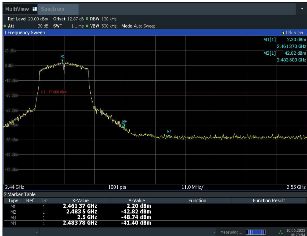
Fig.A.5.6 Band Edges (802.11n-HT20, Ch 1)
