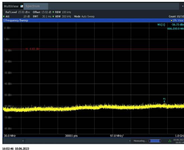
Fig.A.6.1.2 Transmitter Spurious Emission - Conducted (802.11b, Ch1, 30 MHz-1 GHz)
