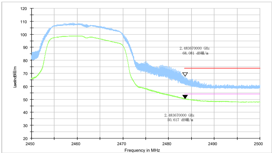
Fig.A.6.2.4 Transmitter Spurious Emission - Radiated (Power): 802.11g, ch11, 2.45 GHz - 2.50GHz
