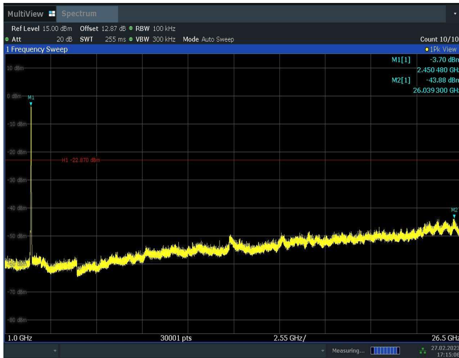
Fig.A.6.1.36 Transmitter Spurious Emission - Conducted (802.11n-HT40, Ch9, 1 GHz-26.5 GHz)
