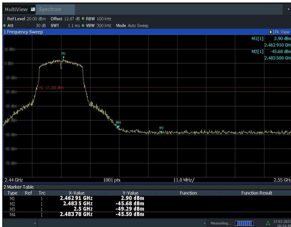
Fig.A.5.4 Band Edges (802.11g, Ch 11)
