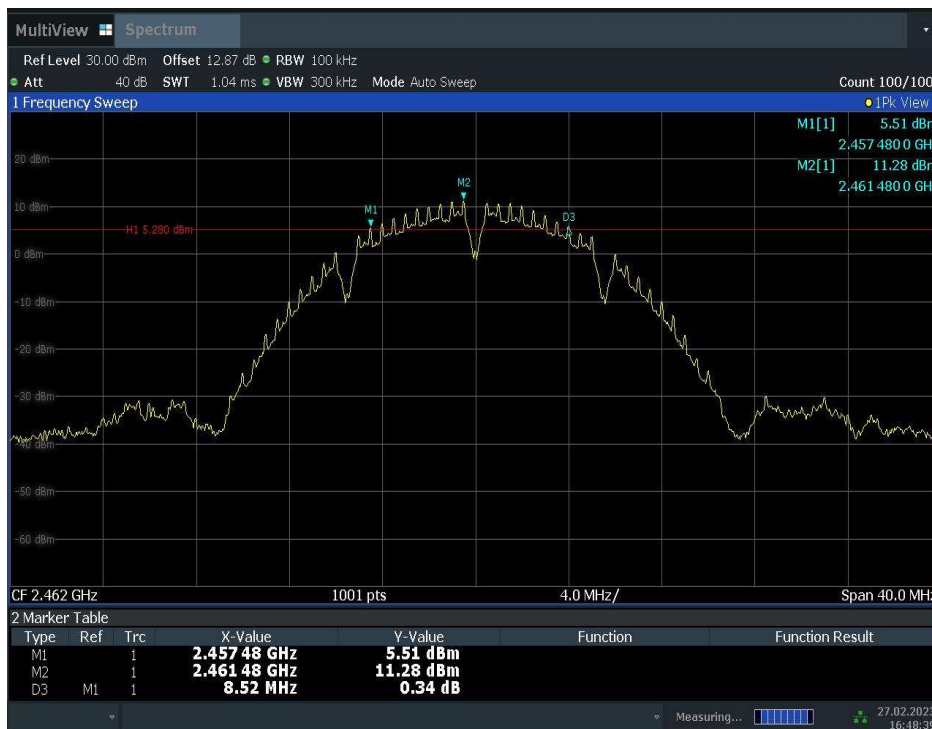
Fig.A.4.3 Occupied 6dB Bandwidth (802.11b, Ch 11)
