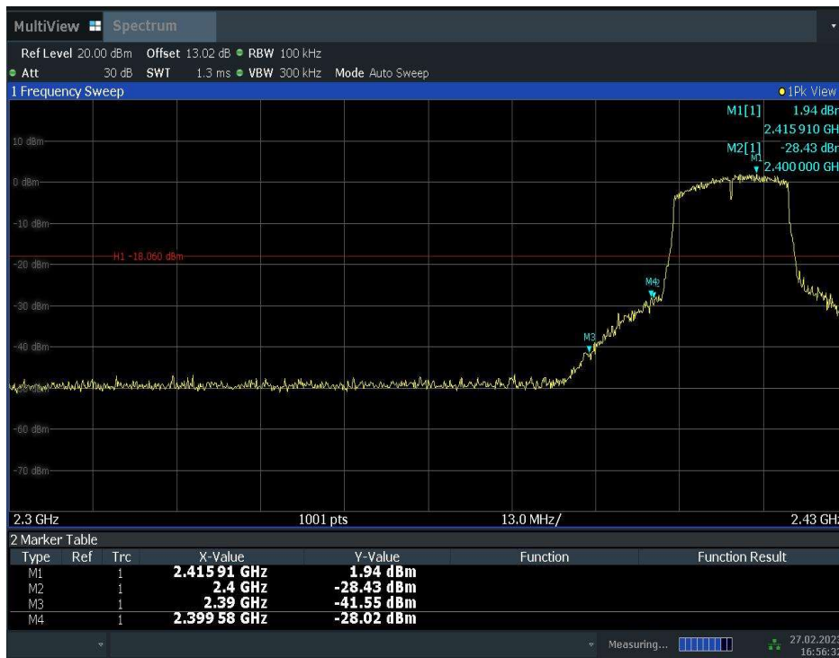
Fig.A.5.5 Band Edges (802.11n-HT20, Ch 1)
