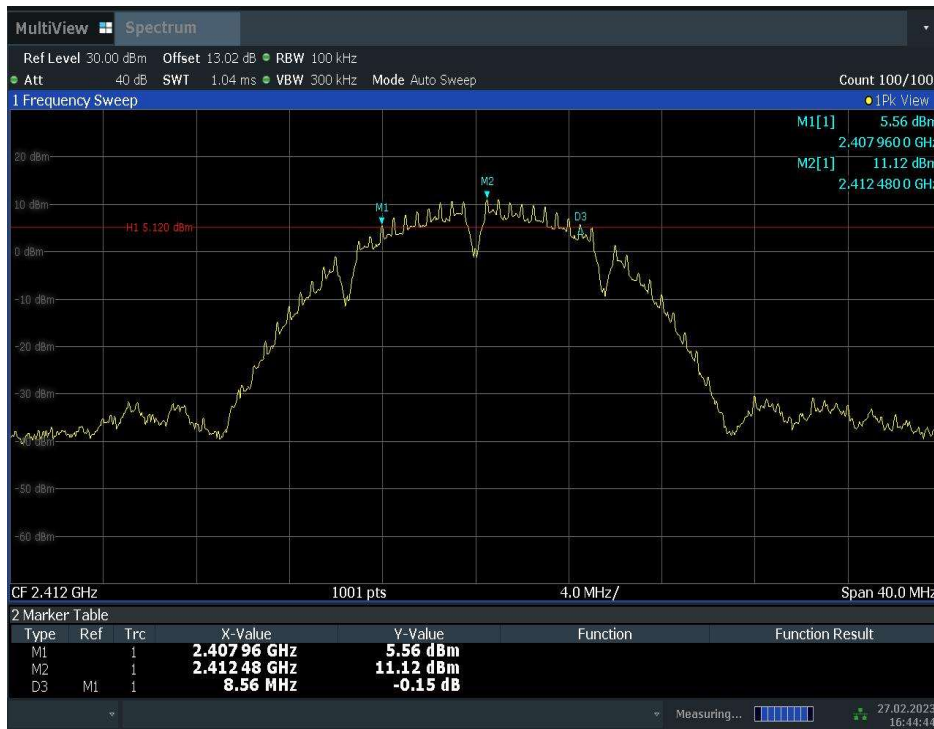
Fig.A.4.1 Occupied 6dB Bandwidth(802.11b,Ch 1)
