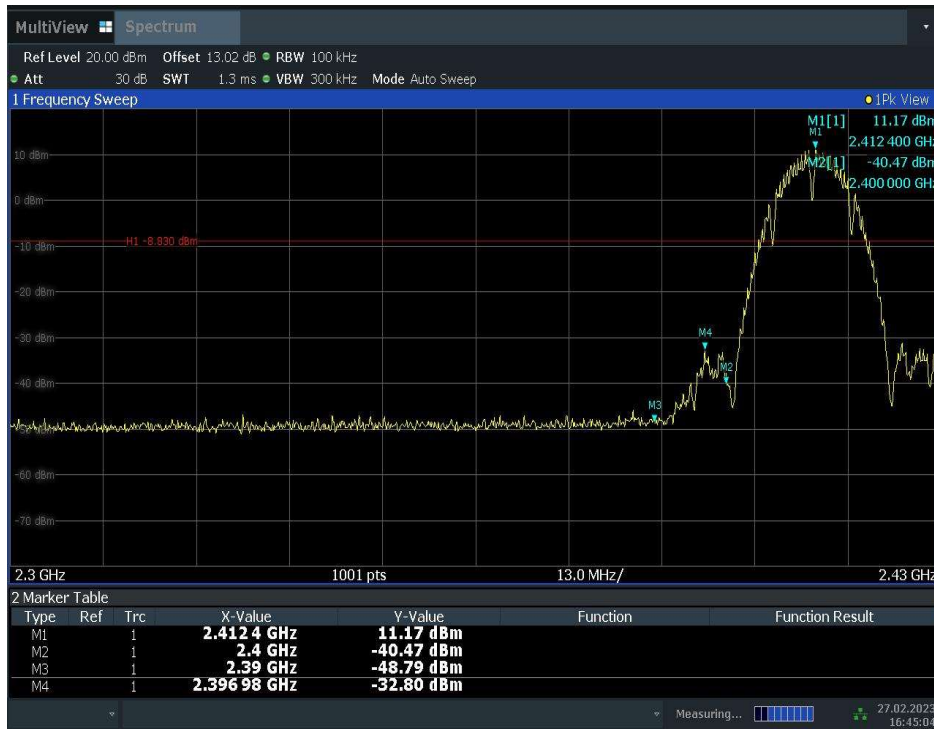
Fig.A.5.1 Band Edges (802.11b, Ch 1)
