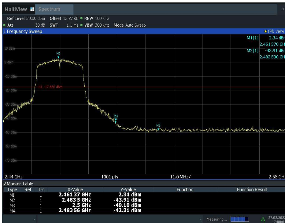
Fig.A.5.6 Band Edges (802.11n-HT20, Ch 11)
