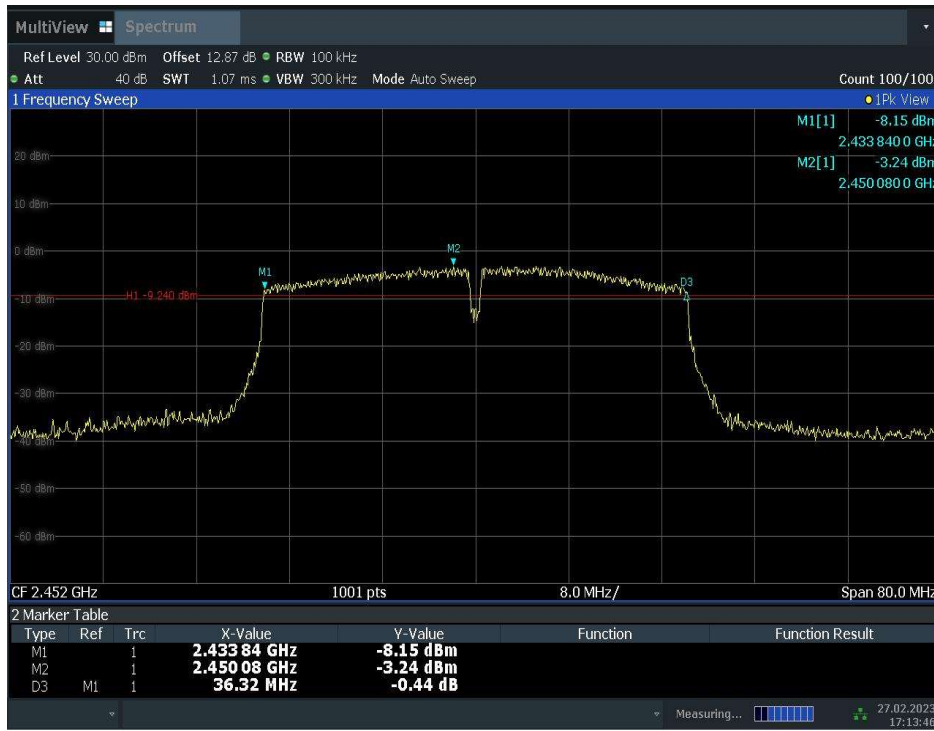
Fig.A.4.12 Occupied 6dB Bandwidth (802.11n-HT40, Ch 9)
