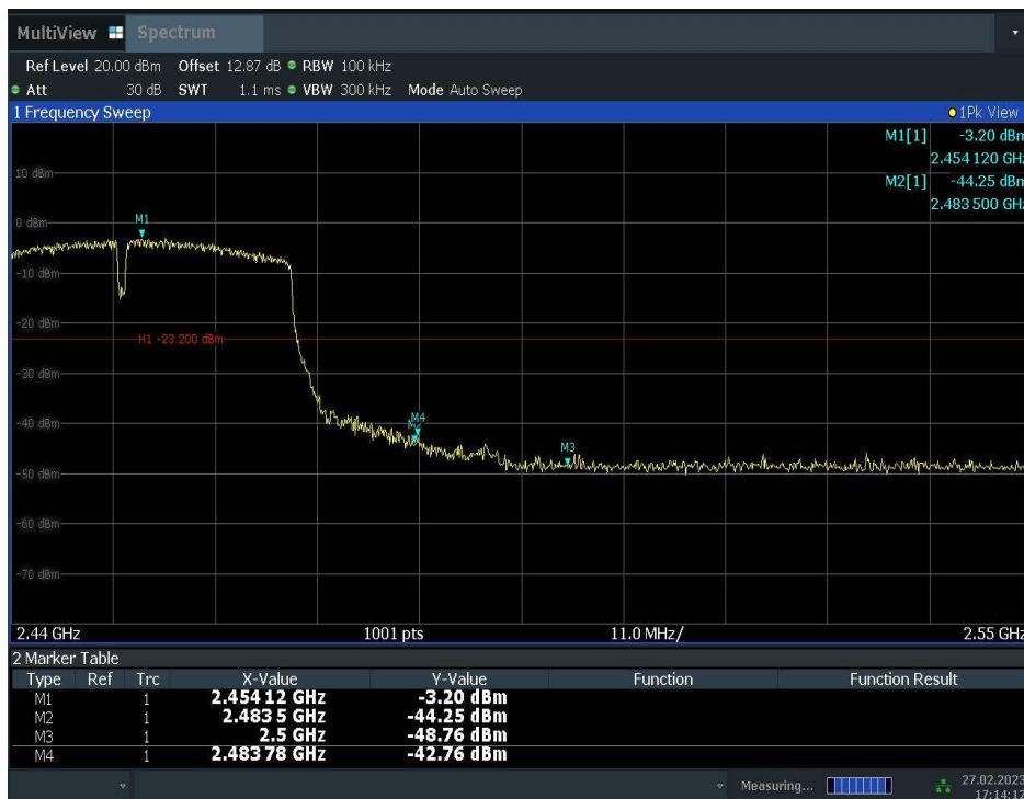
Fig.A.5.8 Band Edges (802.11n-HT40, Ch 9)
