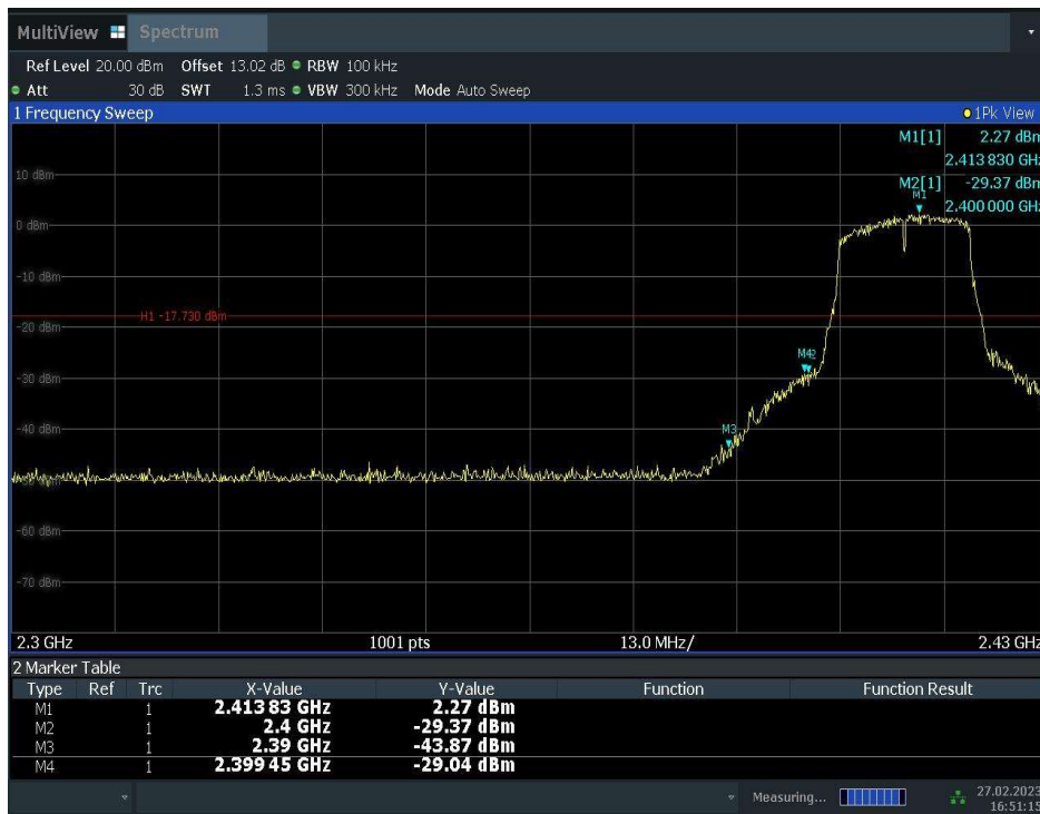
Fig.A.5.3 Band Edges (802.11g, Ch 1)
