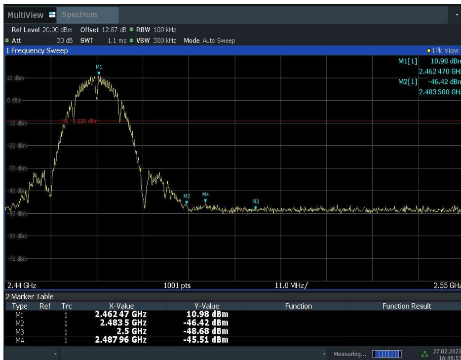
Fig.A.5.2 Band Edges (802.11b, Ch 11)
