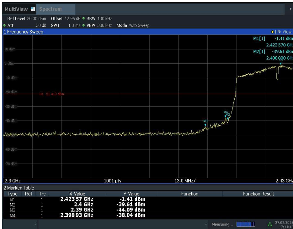
Fig.A.5.7 Band Edges (802.11n-HT40, Ch 3)
