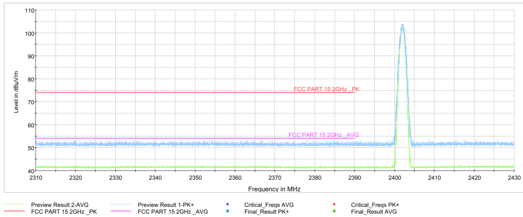
Fig.17. Frequency Band Edges: 8DPSK, Channel 0, 2.31 GHz - 2.45GHz
