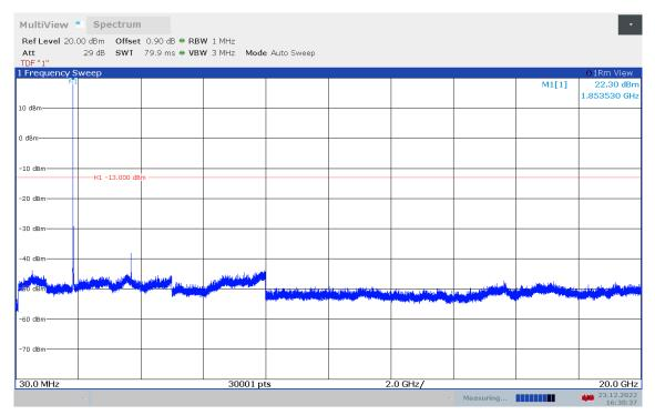
Channel 9400: 30MHz –19.1GHz Spurious emission limit –13dBm.
