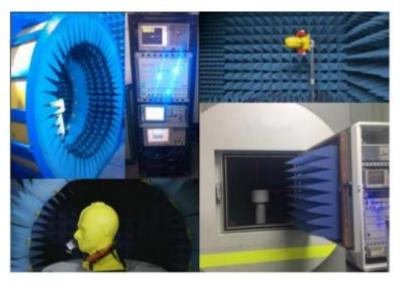
Our company has a number of OTA test darkrooms, ranging from 400MHz to 8.5ghz, which can provide passive test and active test (including OTA overall 2G,3G,4G,5GFR test, WiFi multi-mode test, GPS active test, Bluetooth active test, which can provide antenna gain and efficiency. 2D orientation and apple chart analysis and upper and lower hemisphere efficiency values, mutual disturbance correlation coefficient test items
