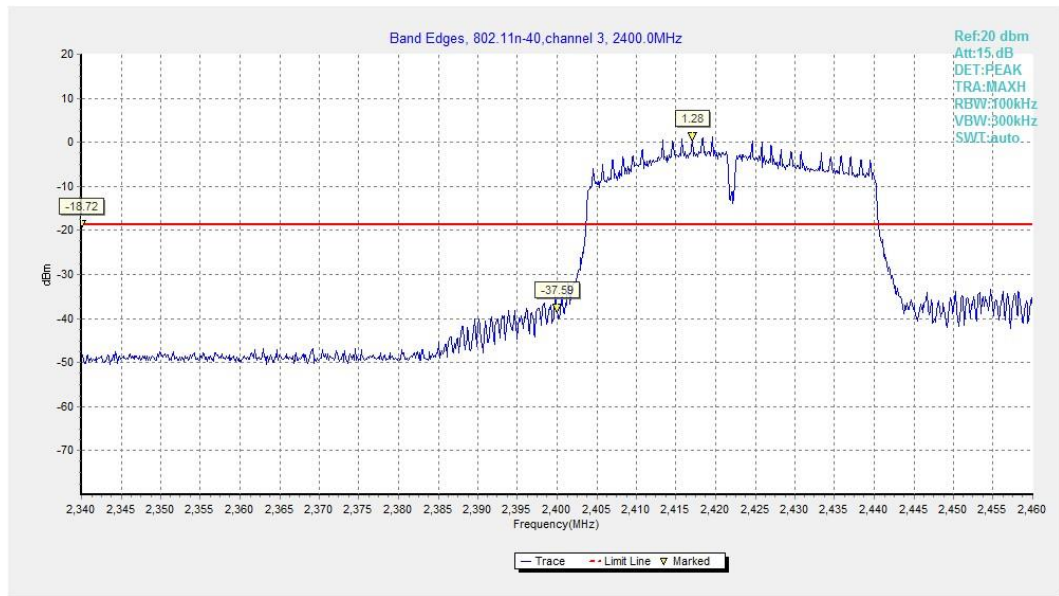
Fig.A.5.7 Band Edges (802.11n-HT40, Ch 3)
