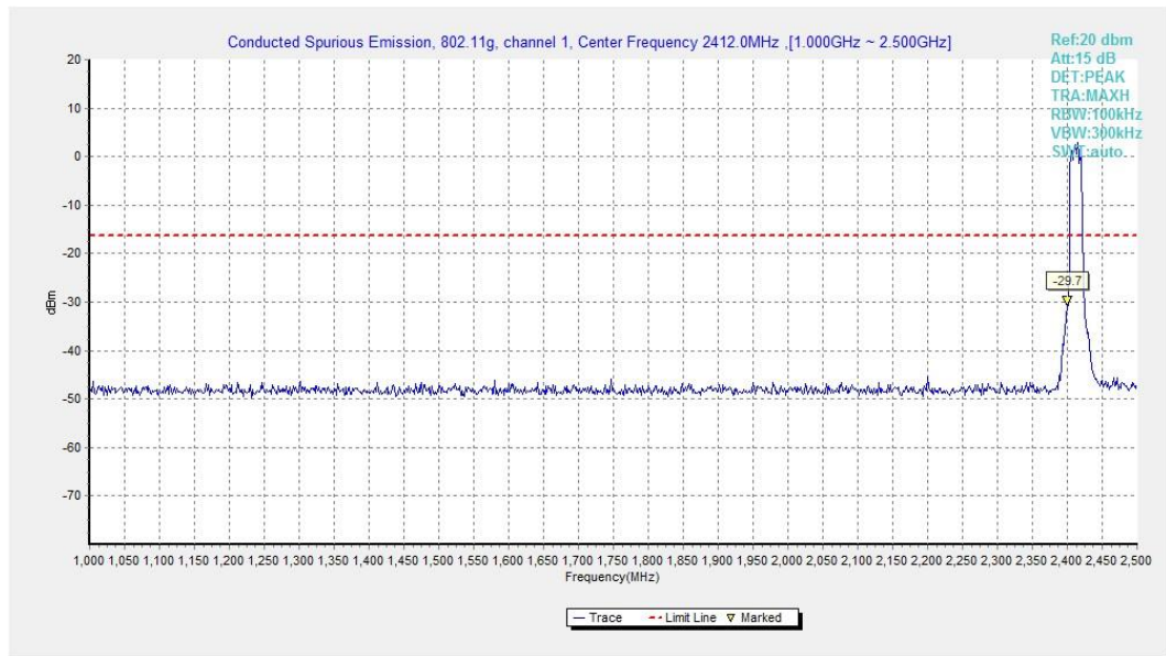
Fig.A.6.1.27 Transmitter Spurious Emission - Conducted (802.11g, Ch1, 1 GHz-2.5 GHz)
