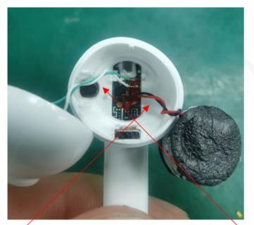
Control the battery wire length of the left ear to 25mm, wrap the battery wire with 4-5 turns, and place the battery pole ear upward The wire length of the battery in the left ear should be controlled as 28mm, and the winding treatment should be done well, and the winding times should be 3-4 turns
