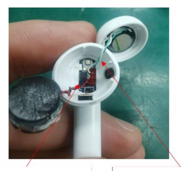
Control the battery wire length of the right ear to 25mm, wrap the battery wire with 4-5 turns
