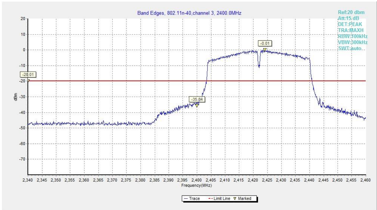
Fig.A.5.7 Band Edges (802.11n-HT40, Ch 3)
