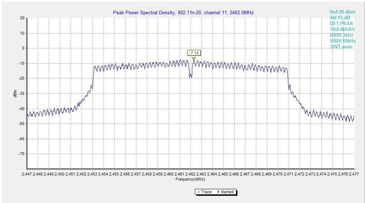
Fig.A.3.9 Power Spectral Density (802.11n-HT20, Ch 11)
