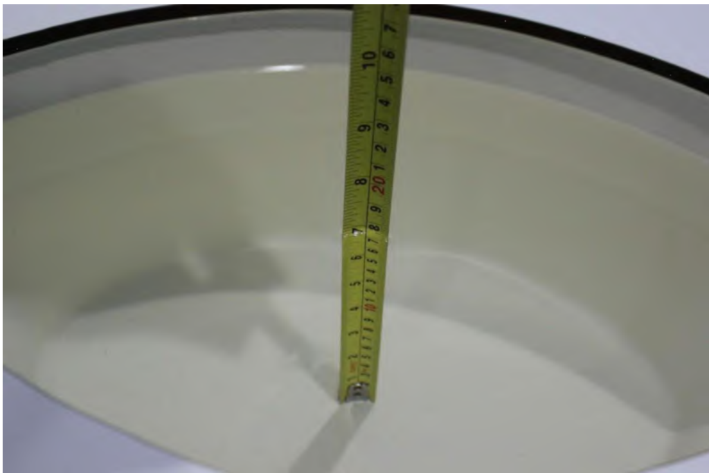
Picture 7-2: Liquid depth in the Flat Phantom(5GHz)
