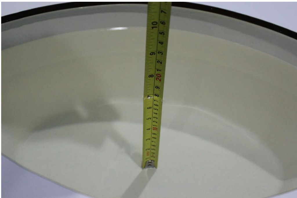
Picture 7-6: Liquid depth in the Flat Phantom (5GHz)
