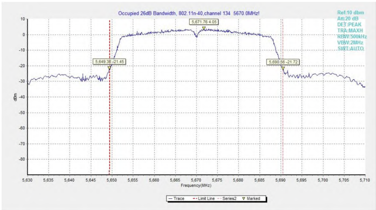
Fig. 15 Occupied 26dB Bandwidth (802.11n-HT40, 5670MHz)
