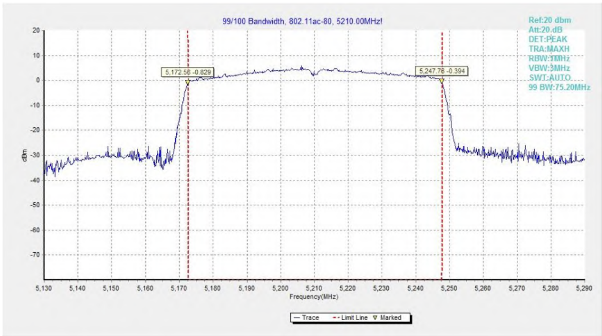
Fig. 45 99% Occupied Bandwidth (802.11ac-VHT80, 5210MHz)
