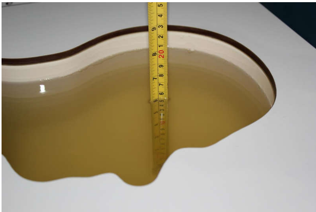
Picture 7-6: Liquid depth in the Head Phantom(2550MHz)
