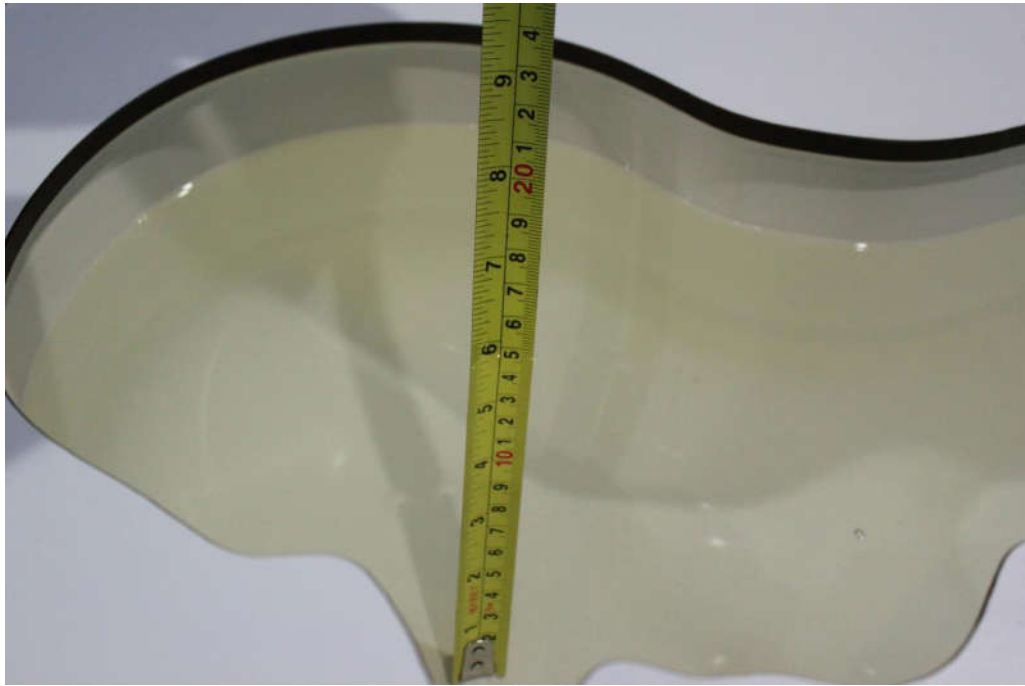
Picture 7-7: Liquid depth in the Head Phantom(5GHz)
