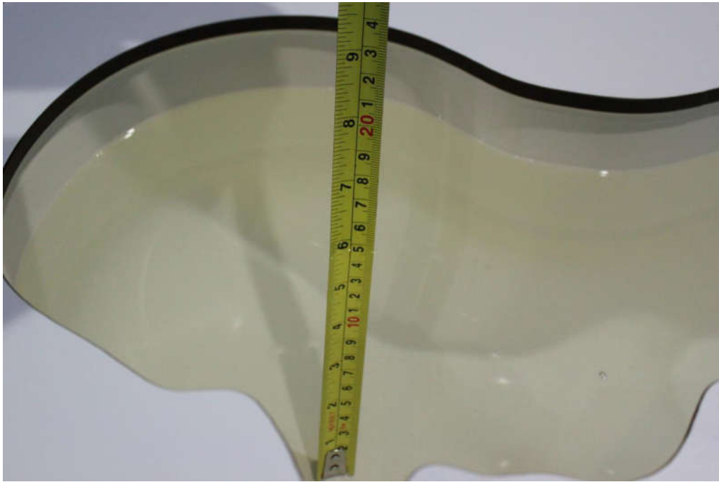
Picture 7-7: Liquid depth in the Head Phantom(5GHz)
