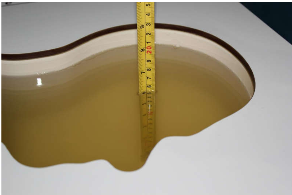
Picture 7-6: Liquid depth in the Head Phantom(2550MHz)
