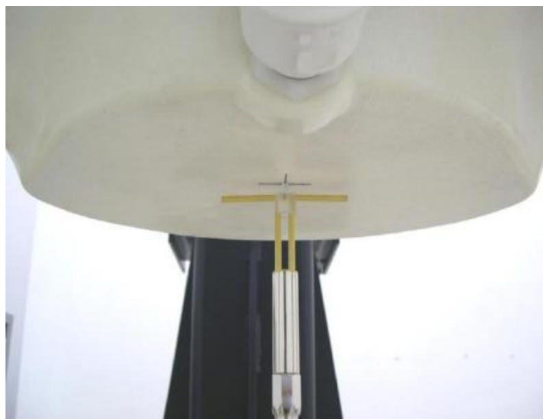
Picture 8.2 Photo of Dipole Setup
