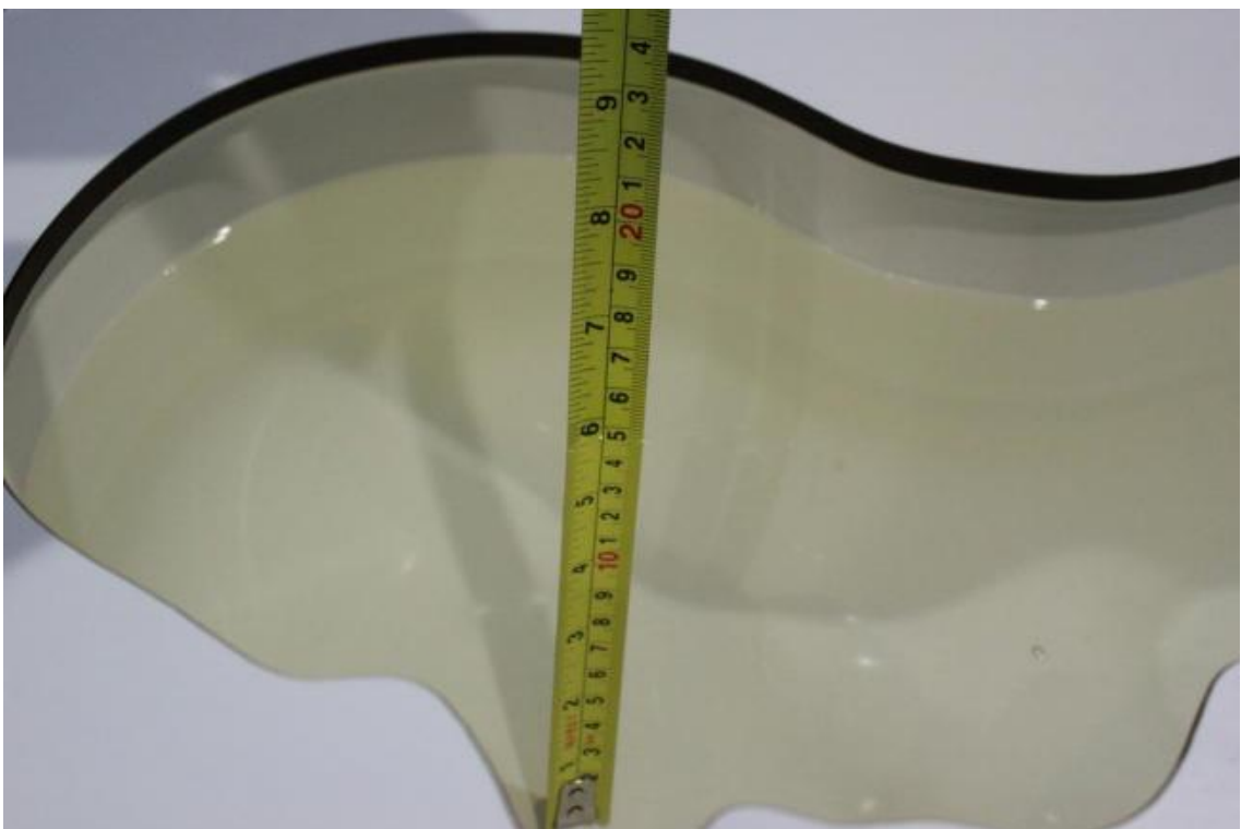
Picture 7-6 Liquid depth in the Head Phantom (5GHz)
