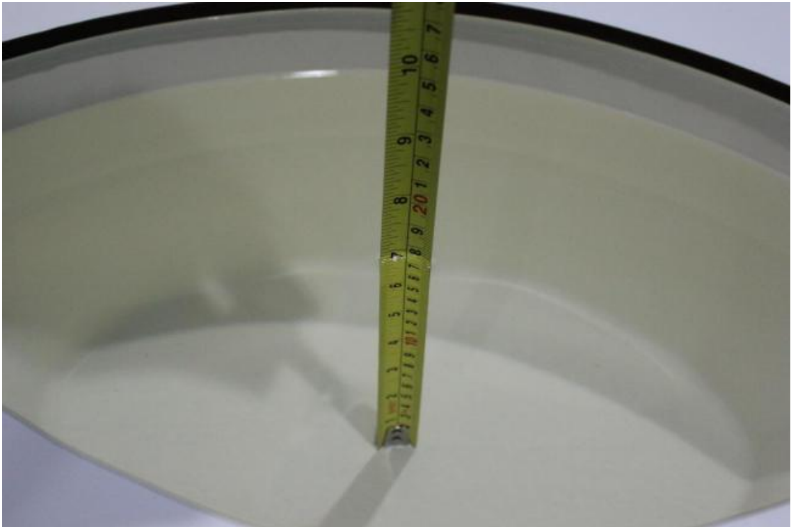
Picture 7-5 Liquid depth in the Head Phantom (3GHz)
