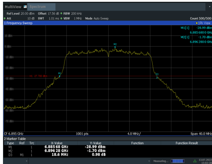
Fig.11 Occupied 26dB Bandwidth (802.11a, 6895MHz)
