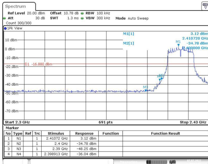
Fig.A.5.3 Band Edges (802.11g, Ch 1)
