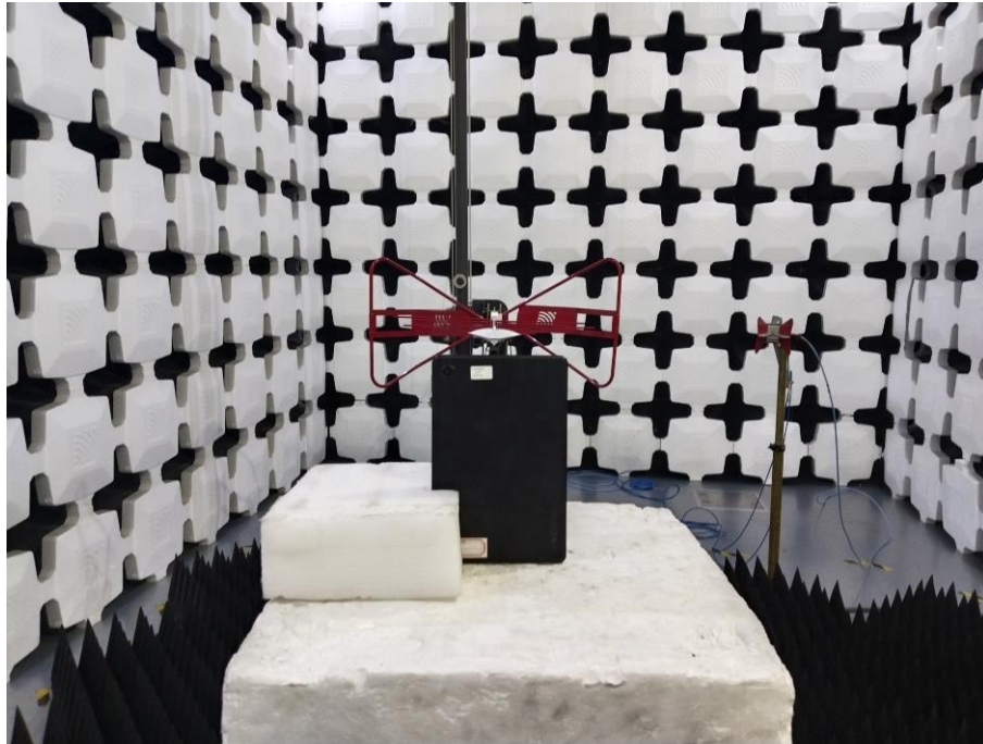
3. Radiated Emissions (Part 15C Wi-Fi/Bluetooth, 1GHz -18GHz)
