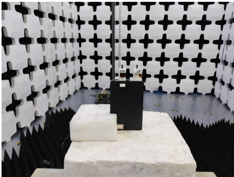
4. Radiated Emissions (Part 15C Wi-Fi/Bluetooth, 18GHz -26.5GHz)
