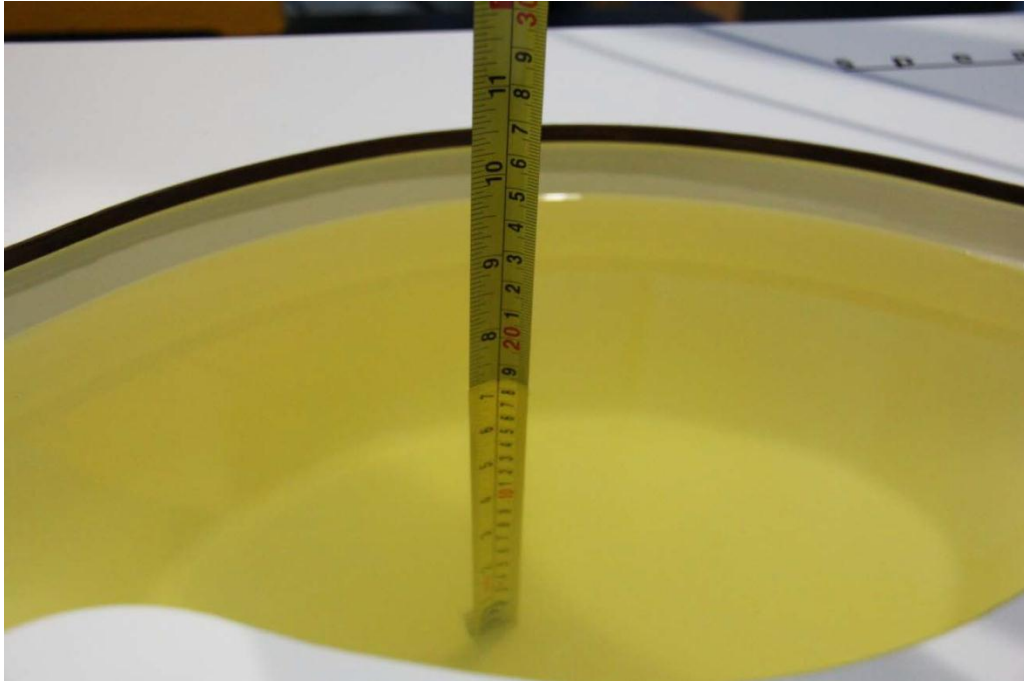
Picture 7-1: Liquid depth in the Flat Phantom(2450MHz)
