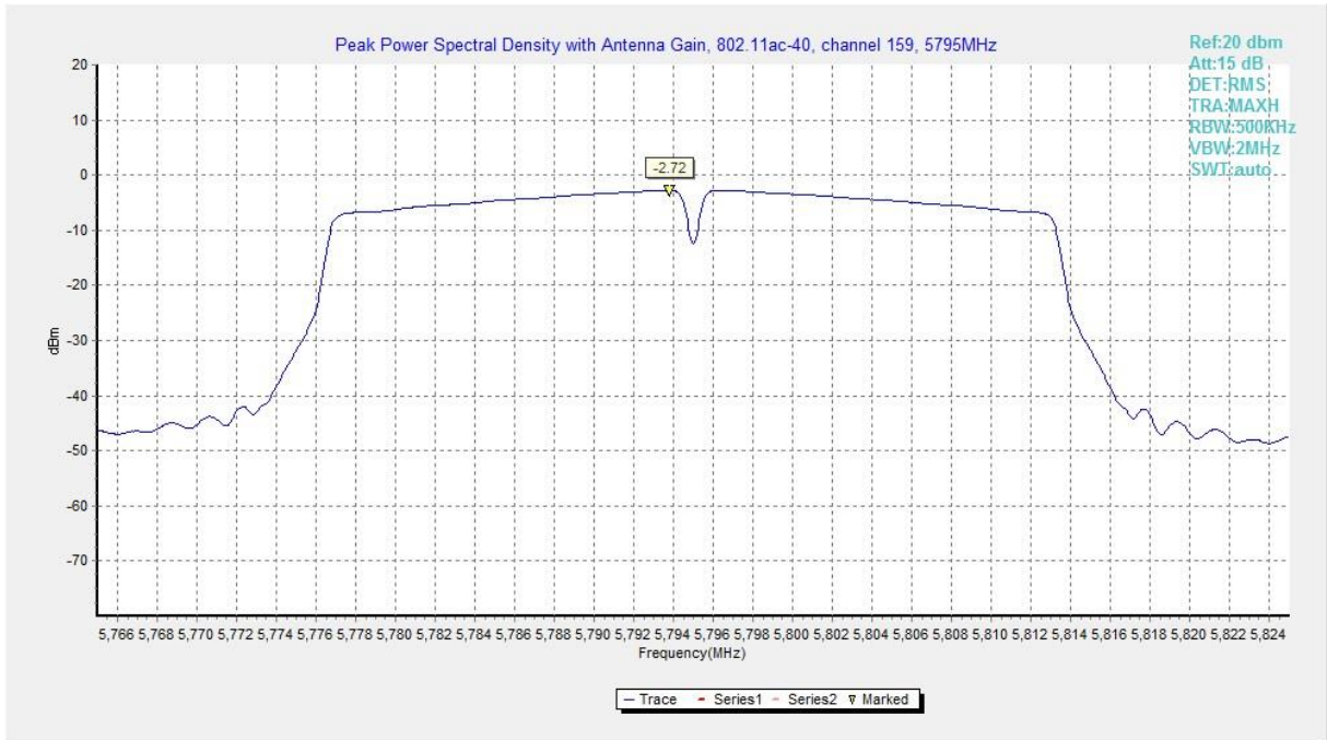
Fig. 8 Occupied 6dB Bandwidth (802.11ac-HT40, Ch 159)
