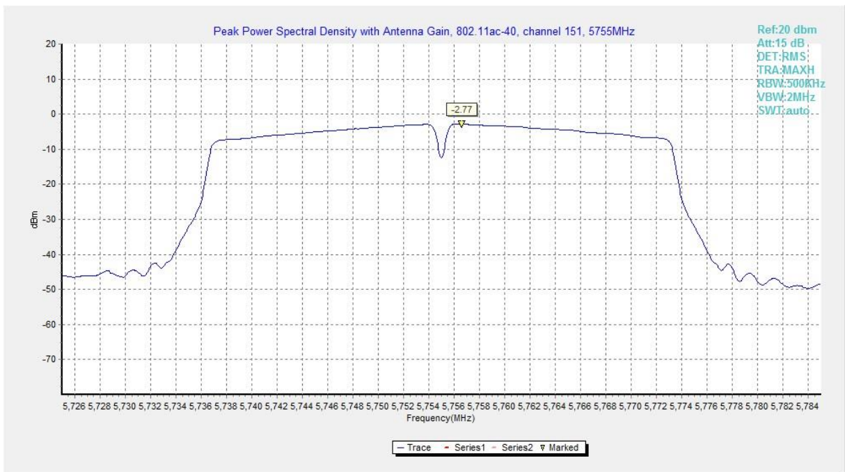
Fig. 7 Occupied 6dB Bandwidth (802.11ac-HT40, Ch 151)
