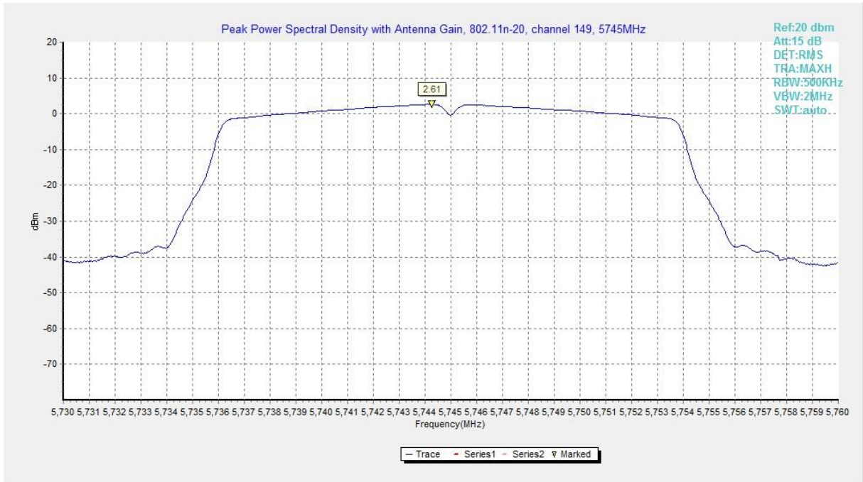
Fig. 4 Occupied 6dB Bandwidth (802.11n-HT20, Ch 149)
