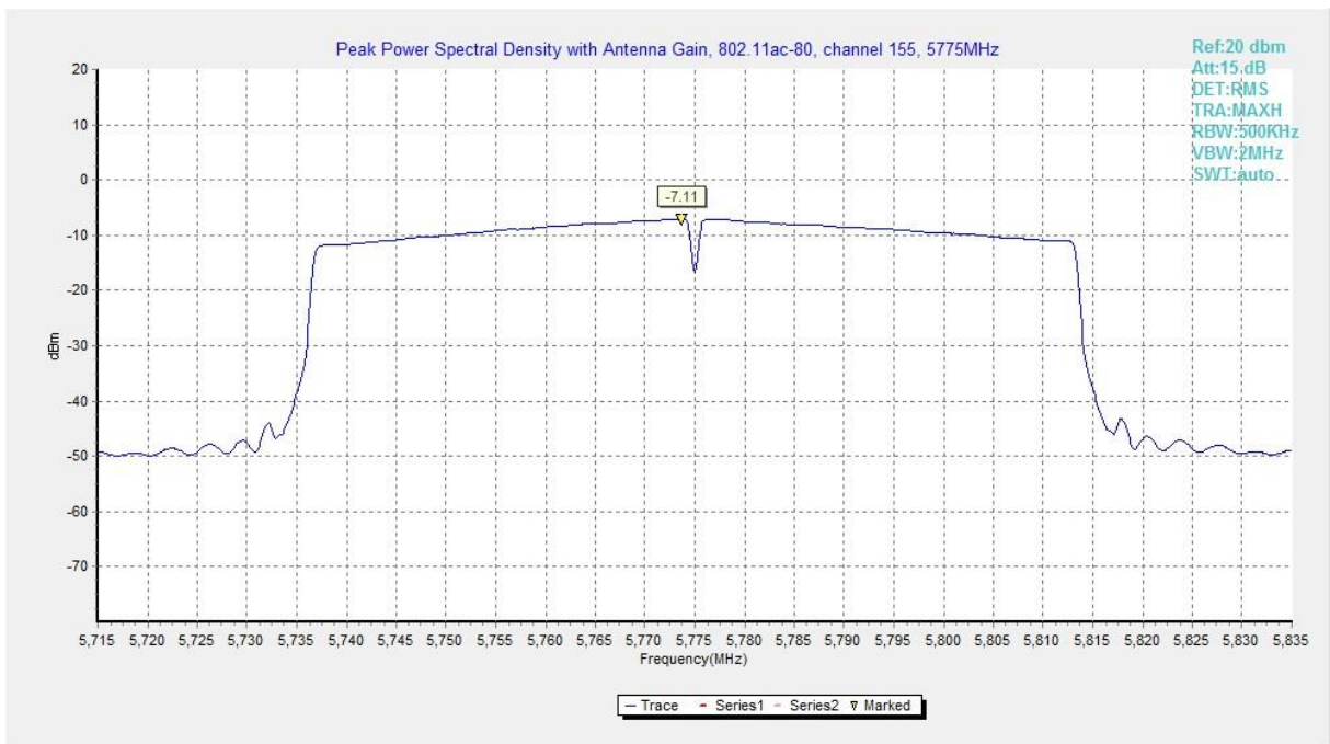
Fig. 9 Occupied 6dB Bandwidth (802.11ac-HT80, Ch 155)
