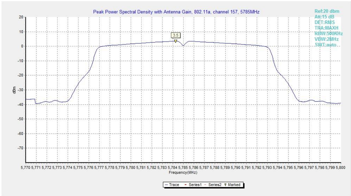
Fig. 2 Occupied 6dB Bandwidth (802.11a, Ch 157)
