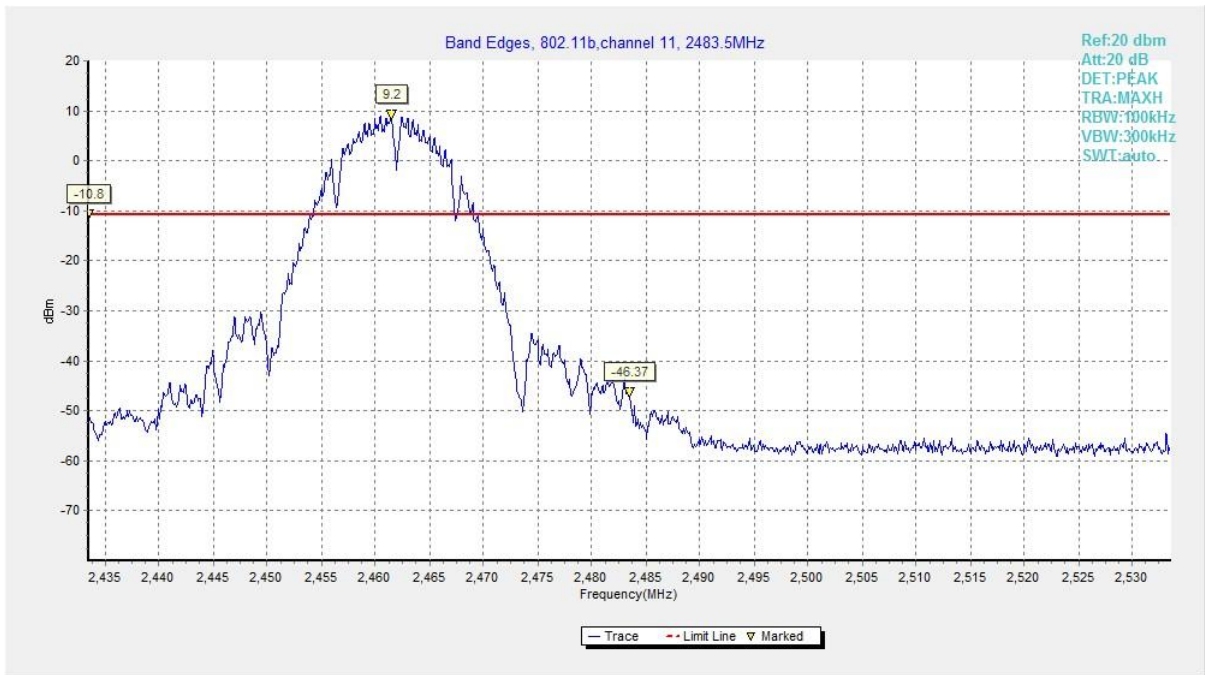
Fig.26 Band Edges (802.11b, CH 11)
