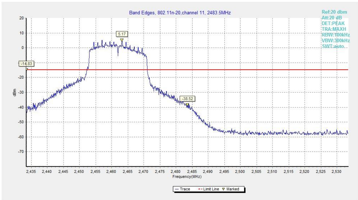
Fig.30 Band Edges (802.11n HT20, CH 11)
