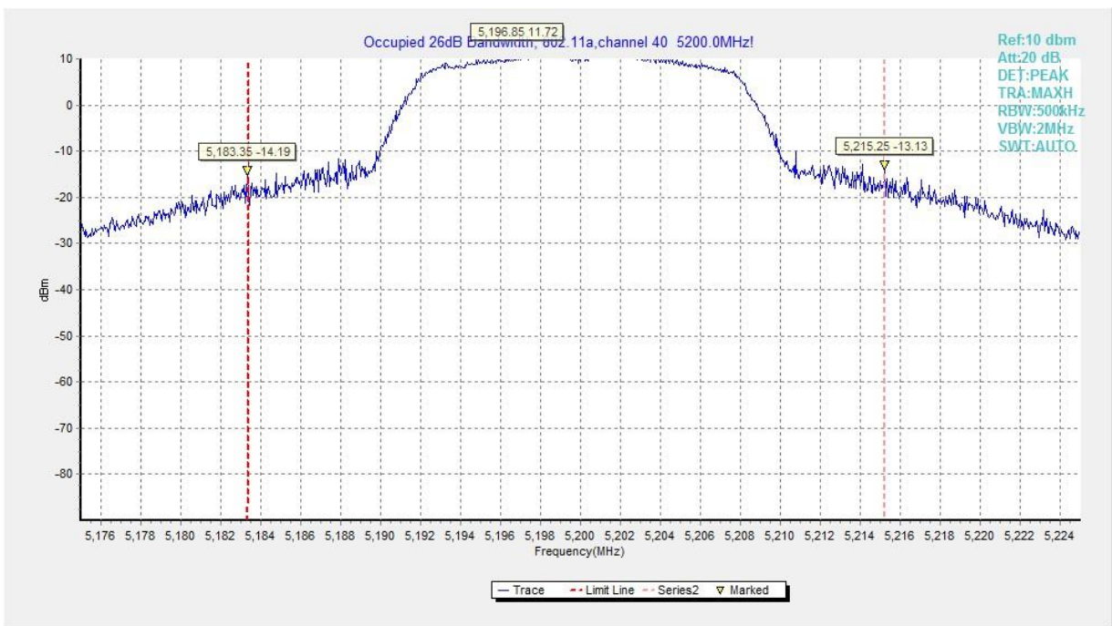
Fig. 2 Occupied 26dB Bandwidth (802.11a, 5200MHz)
