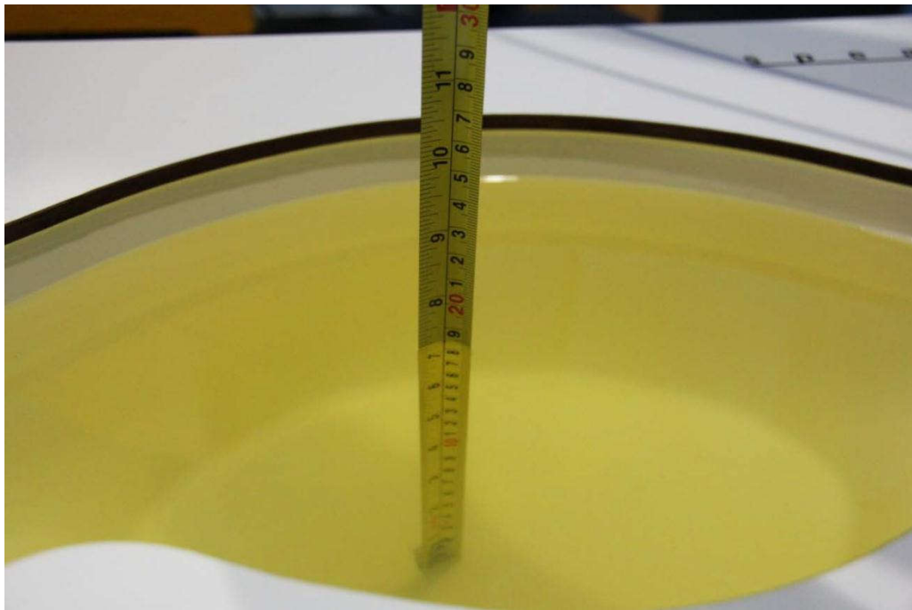
Picture 7-5: Liquid depth in the Flat Phantom (2300MHz)
