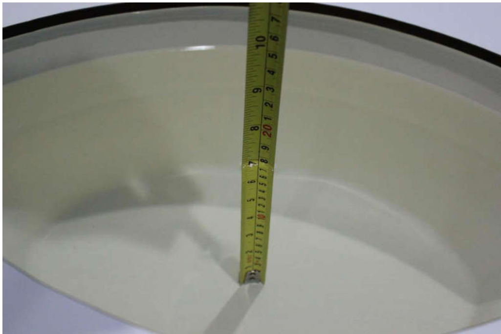
Picture 7-8: Liquid depth in the Flat Phantom(5GHz)
