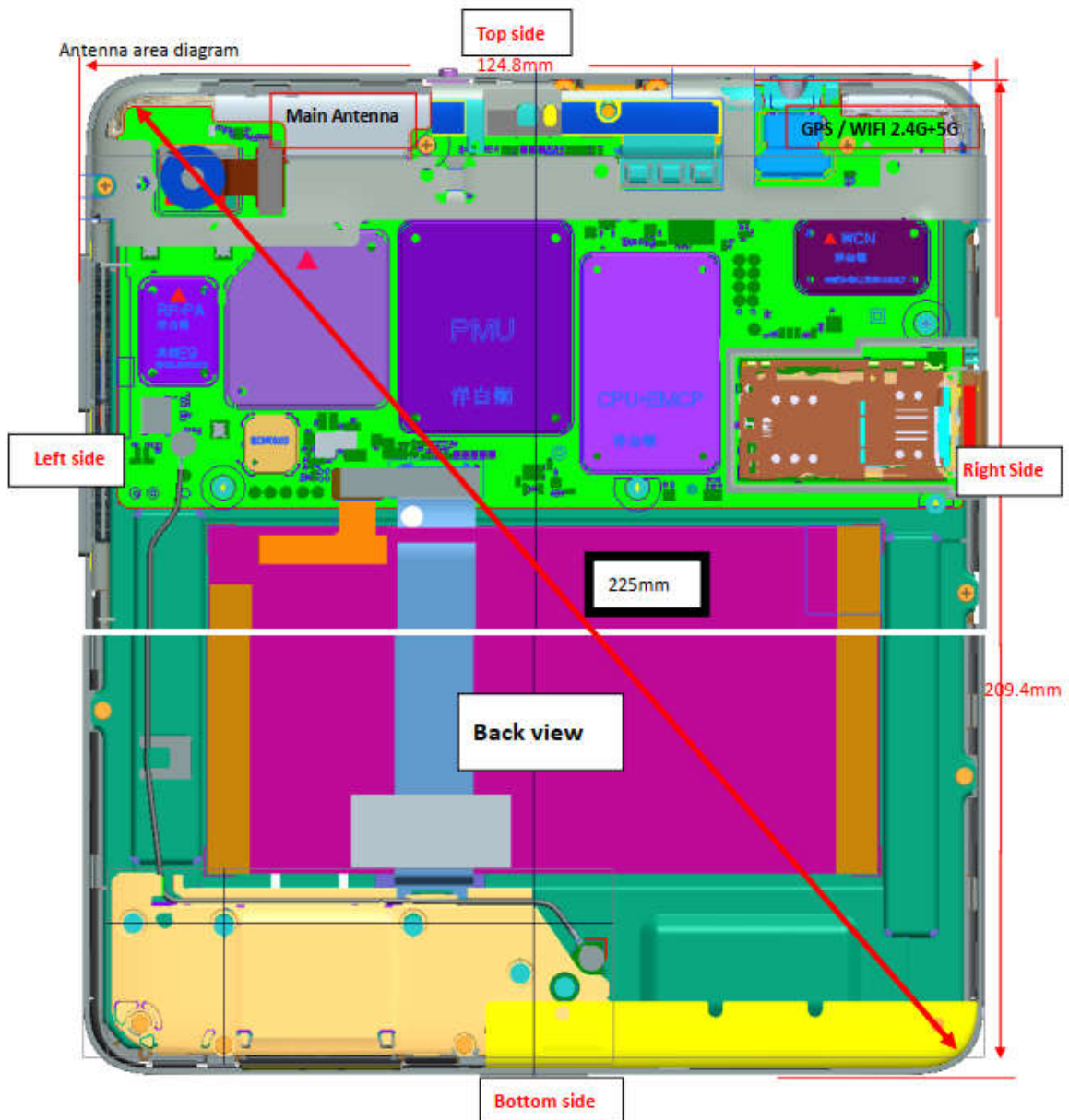
Picture 11.1 Antenna Locations (Back View)
