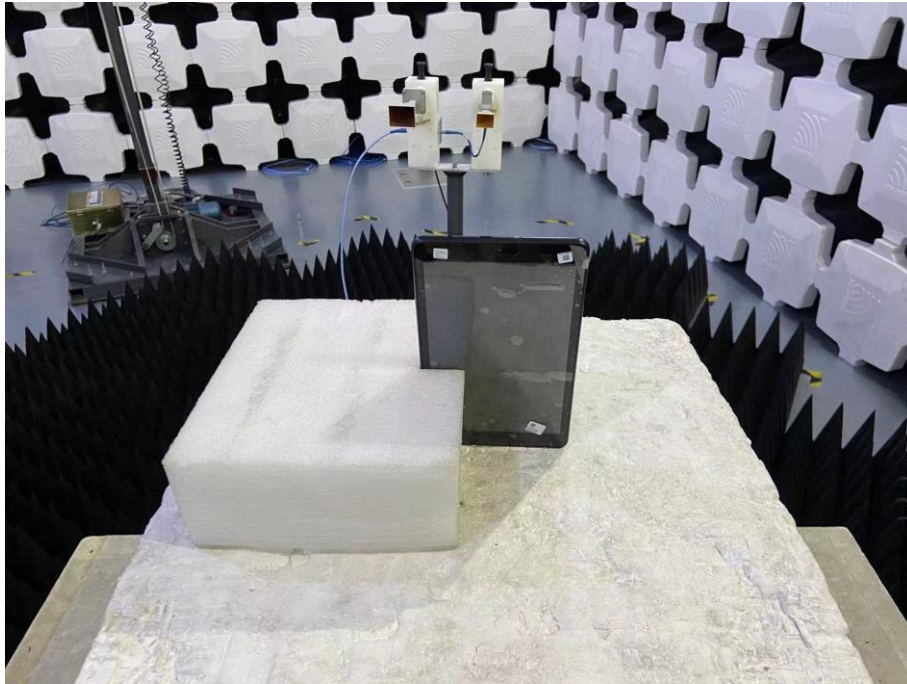
17. Radiated Emissions (Part 15C, 26.5GHz -40GHz)
