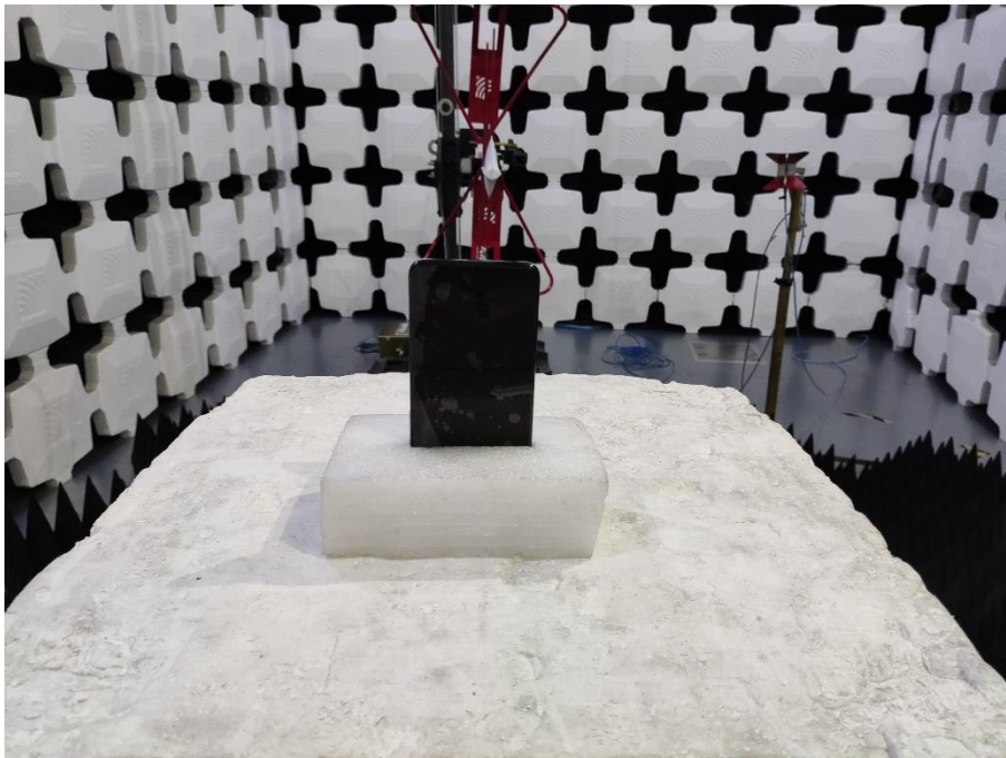
18. Radiated Emissions (Part 22/24/27, 30M-18GHz)
