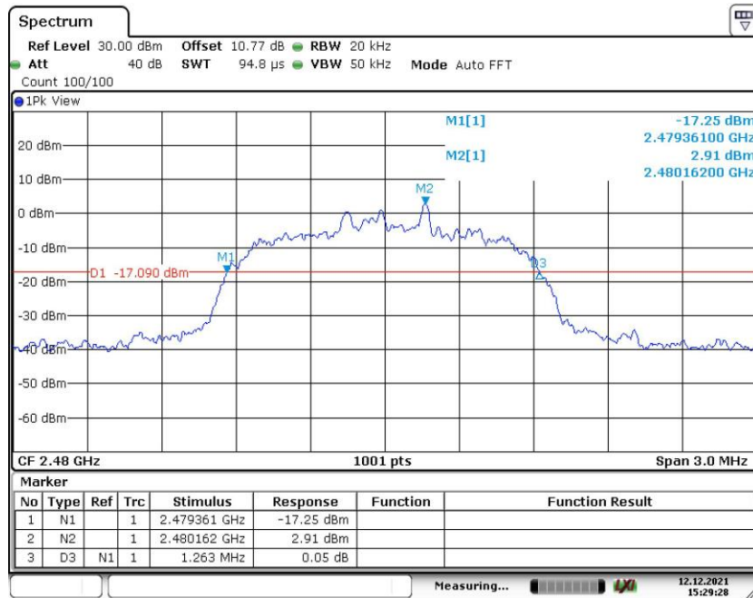
Fig. 75 20dB Bandwidth (8DPSK, CH78)
