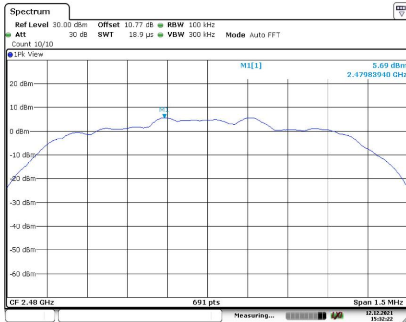
Fig. 37 Conducted Spurious Emission (8DPSK, CH78, 2.480GHz)
