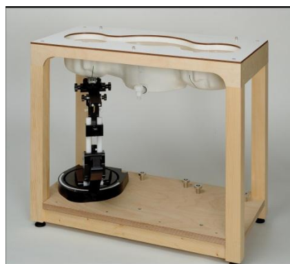
Picture C.8: SAM Twin Phantom
